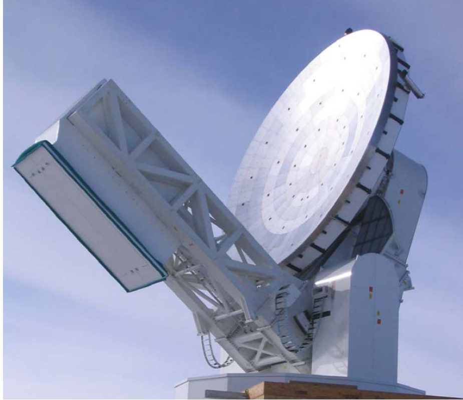
Figure 1.28: The SPT under construction. Image credit: Steve Padin
