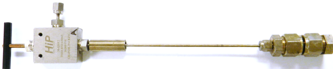
Figure 3.2. 4.1 mL Swagelok® batch reactor with gas sampling valve
