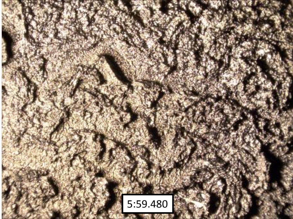
Figure 6.18: Image of deposit layer just after alcohol-induced collapse (time interval is listed as min:sec.msec)
