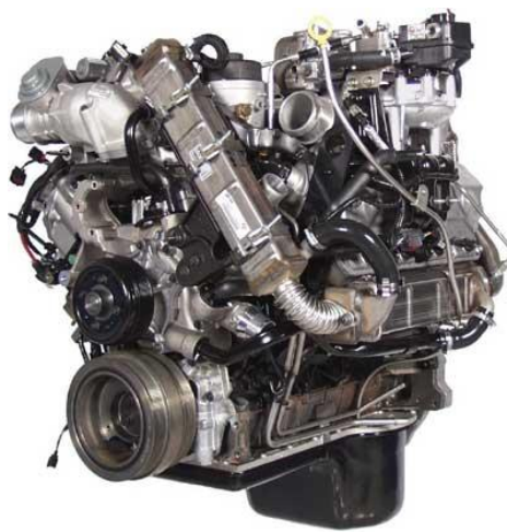
Figure 2.13: 6.4L diesel engine
