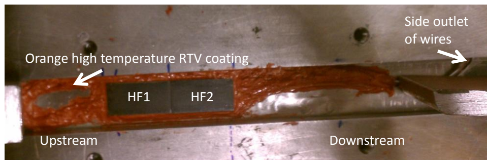
Figure 2.12: Actual heat flux probe installation
