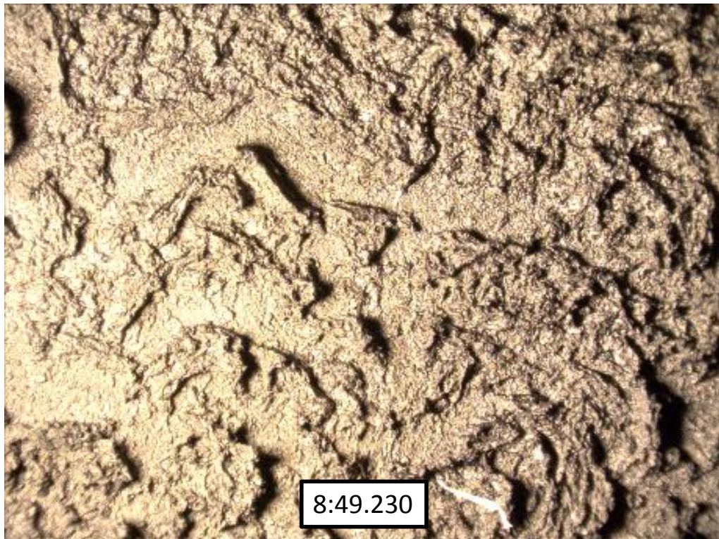
Figure 6.19: Image of contracted deposit layer (time interval is listed as min:sec.msec)
