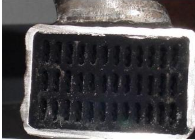
Figure 1.1: Cross section of a fouled diesel EGR cooler [6]
