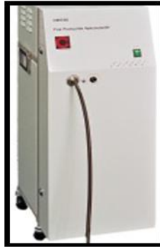
Figure 2.16: Cambustion differential mobility spectrometer (DMS500)
