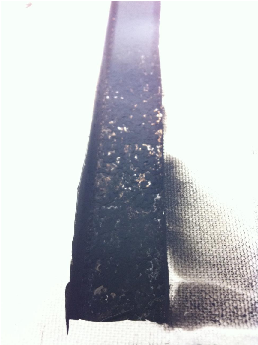
Figure 7.17: Image of deposit surface after water condensation from exhaust gas
