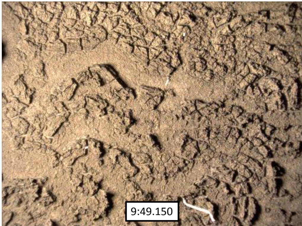
Figure 6.21: Image of contracted and mud-cracked deposit layer (time interval is listed as min:sec.msec)
