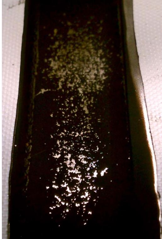
Figure 7.20: Deposit surface spallation resulting from angled airflow
