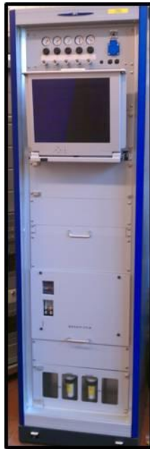
Figure 2.15: AVL SESAM emissions analyzer
