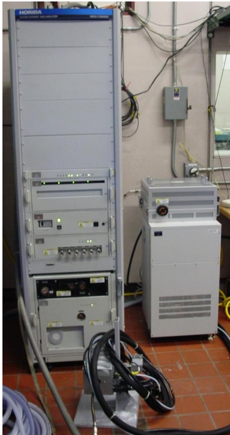
Figure 4.3 – Horiba Mexa7100DEGR emission analyzer bench
