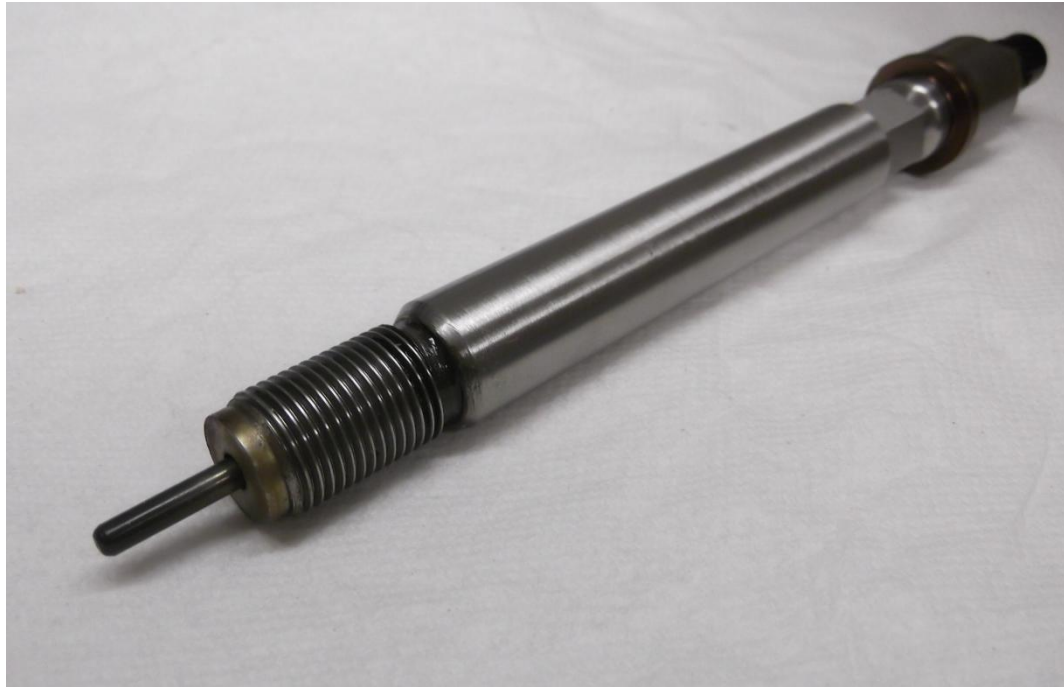
Figure 8.3 – Centrally mounted sleeve adapter with the glow plug installed
