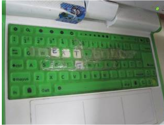
Figure 3.2: Broken OLPC Push-Membrane Keyboard.
