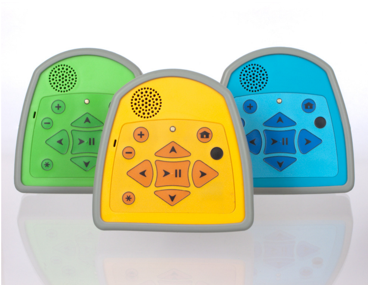
Figure 2.9: The Talking Book: A state-of-the-art Rural Audio Computer designed specifically for on-demand information access in developing regions. To access audio content, end users navigate through voice prompts using the small number of input buttons visible on the device.
