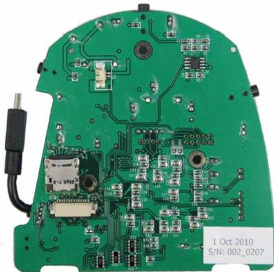
Figure 2.14: Literacy Bridge's Talking Book with its 152 commercial off-the-shelf components (Back Side).
