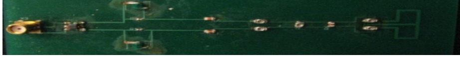
Figure 3.5: The dual-resonator tank and its matching network. The two loops on the right act as coils for tanks.
