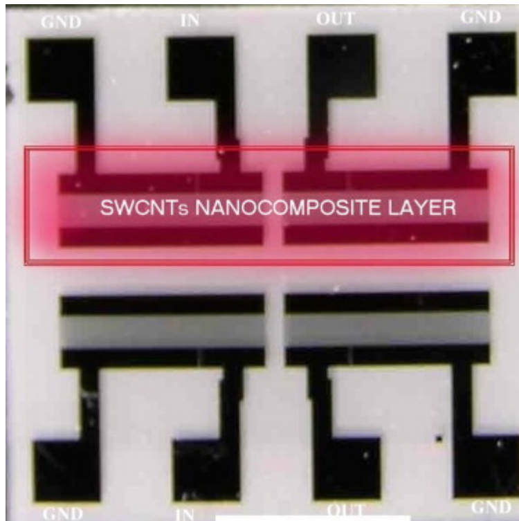
Figure 1-12 Image of two SAW sensors with carbon nanotube piezoelectric delay line. Reprinted with permission from 89 . Copyright Elsevier.
