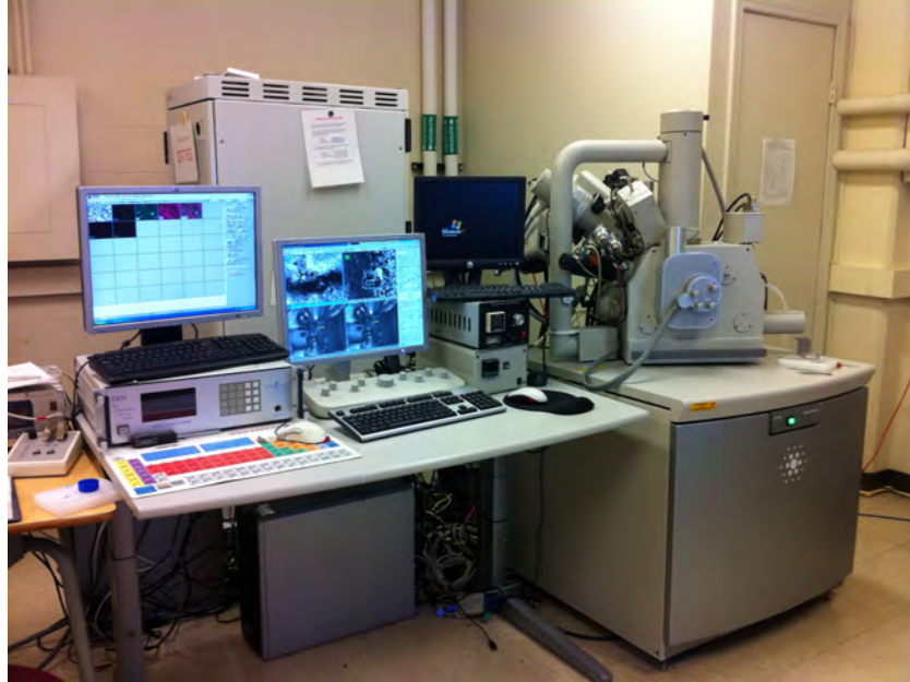
Figure 1. FEI Quanta 200 3D Focussed Ion Beam Workstation and Environmental Scanning Electron Microscope
