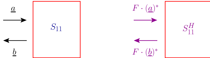
Figure 3.3: The relationship between wavefronts in a medium that exhibits reciprocity. Reciprocity tells us that S_{11}^H \cdot \underline{a} is obtained by time-reversing the wave before and after sending \underline{a} into the medium, and we call this sequence of operations double phase conjugation .
