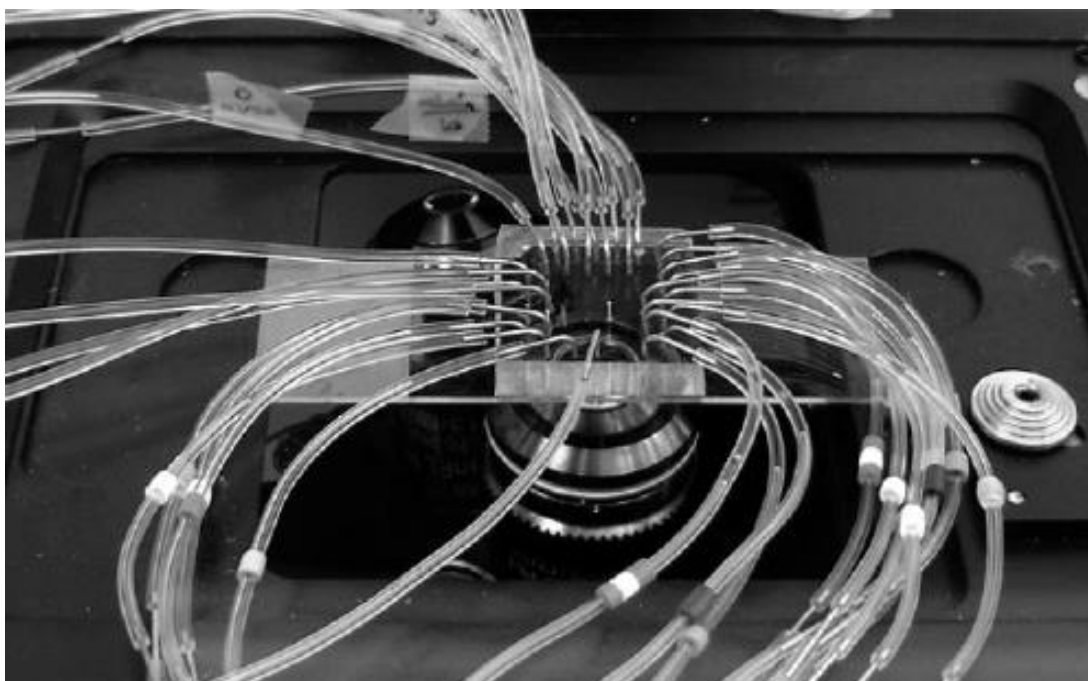
Fig. A.10 With each additional operation in syringe-driven LOC devices, more supportive equipment is necessary (each tube is typically connected to a syringe pump not pictured). With complicated LOCs, it becomes increasingly difficult to integrate with also complicated optics due to spatial limitations [37].
