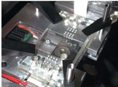
Fig. B.7 A) Microfluidic device used to analyze embryo metabolism. 82 External tubing used for pneumatics or syringe driven inlets can be cumbersome and problematic for clinical application B) Microfluidic device used to culture embryos, while simultaneously permitting assessment of glucose utilization as a means of non-invasive embryo assessment on the same device. 81 Clinical usability is preserved by using a preprogrammed Braille display to drive flow.
