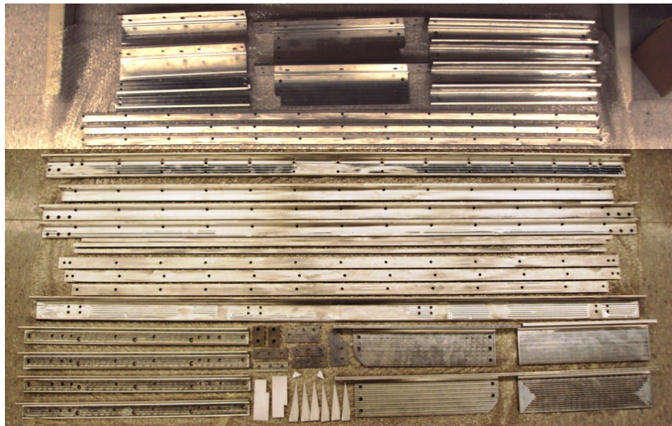
Figure A.4: A snapshot of all test section pieces machined by QuickParts prepared for assembly.
