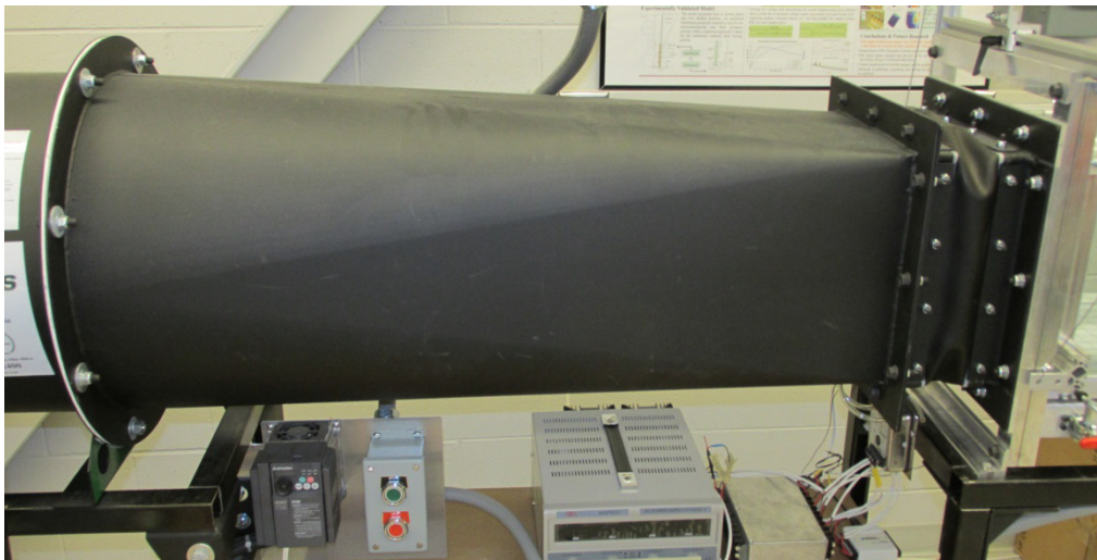
Figure A.10: A snapshot of the diffuser section installed on the wind tunnel assembly and ready for operation.
