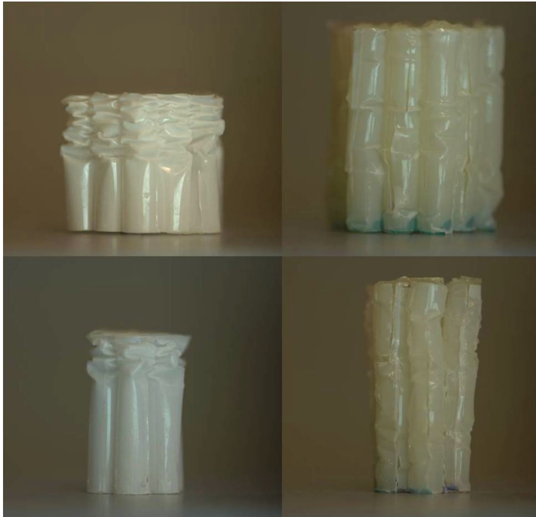
Figure 5.11: The images comparing the deformations of filled and unfilled 7-cell and 19-cell honeycombs. The unfilled specimens are shown on the left column and the filled specimens on the right column. Notice the progressive localized failure spread over a continuous region in the unfilled specimens. In contrast, the localized folds in the filled specimens occur in a random fashion. Longitudinal tearing is seen in both the filled honeycombs. In the filled 7-cell specimen, notice some global deformation that is not present in the filled 19-cell specimen due to lower aspect ratio.
