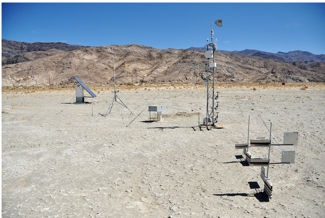
Figure 3.2: View of the ACI project site at Owens Lake, facing east. The system includes, from left, the solar power system, tower 2, electronics box, tower 1, and the BSNE collection array.
