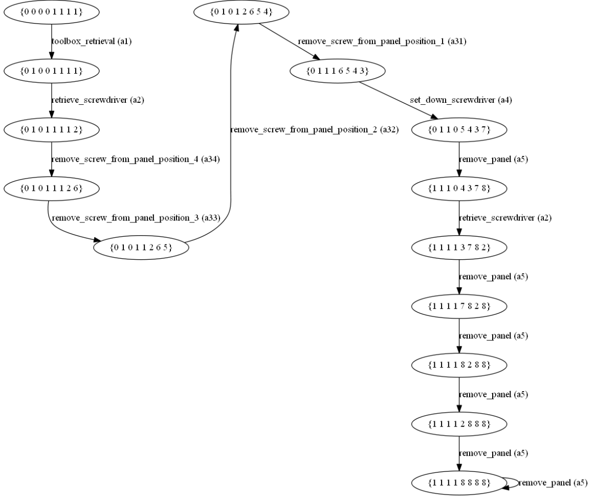
Figure 5-3: State evolution for the optimal MDP policy, case 4b (4 goals, n_h=4 ), starting from s^i = \{\text{no goals set, all actions in history } toolbox\_retrieval (a_1)\} , for s^i = \{g_1^i, g_2^i, g_3^i, g_4^i, a_1^i, a_2^i, a_3^i, a_4^i\}
