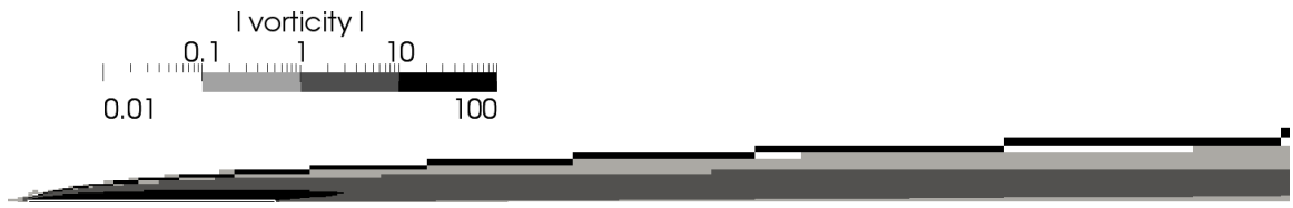
Figure 4.5: The magnitude of the vorticity field for the Re = 2000 / 0 case with the plate outlined in white and the \delta -boundary also colored in black, from x/c = 0.0 to x/c = 5.0 .
