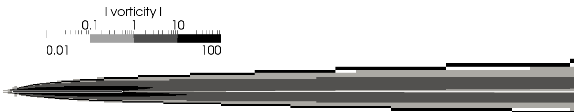
Figure 4.7: The magnitude of the vorticity field for the Re = 2000 / 4000 case with the plate outlined in white and the \delta -boundary also colored in black, from x/c = 0.0 to x/c = 5.0 .
