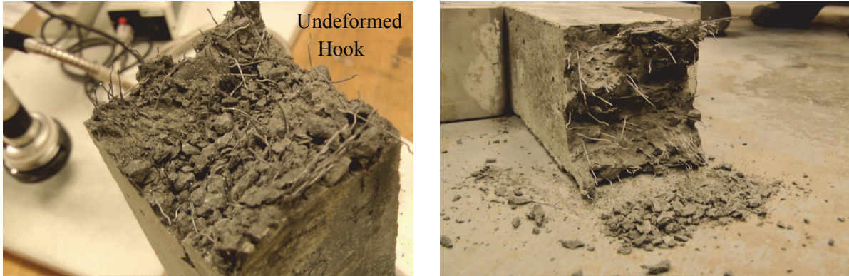
Figure 3.9: Pronounced matrix spalling evident in large dogbone breaks
