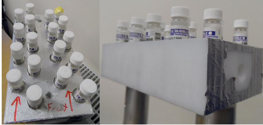
Figure 4.27: Photographs of the top and side of the pion detector setup used on the ASTRA-GEMINI experiment. The bulk of the bubble detector gel is inside the block and the rod is protected on the sides from contaminant (\gamma, n) neutrons.
