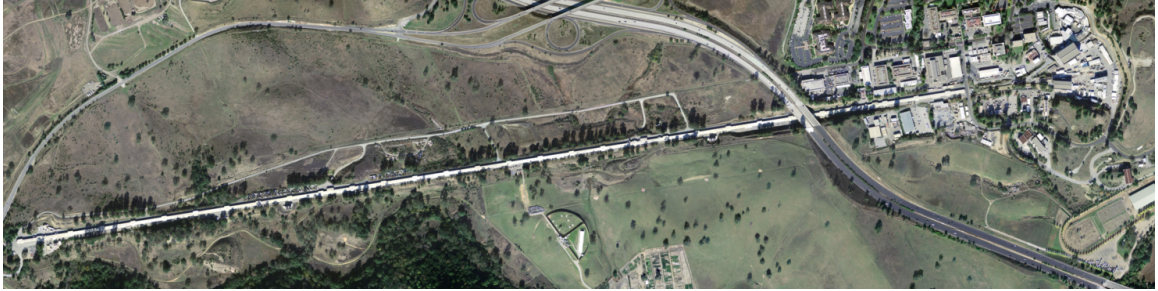
Figure 1.1: Aerial photograph of the SLAC 3 km long linear accelerator. Note the I-280 expressway crossing over the facility for a sense of scale.
