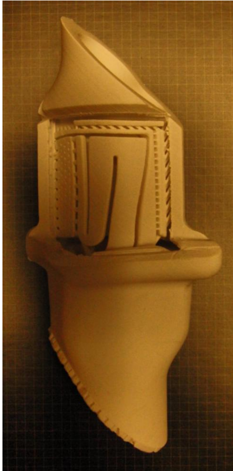
Figure 1.9 Integrally cored mold with side wall cut away to view the core. The external walls define the shape of the airfoil while the interior core defines the cooling passages in the cast airfoil. This was built at a 45° angle from the vertical direction of the image.
