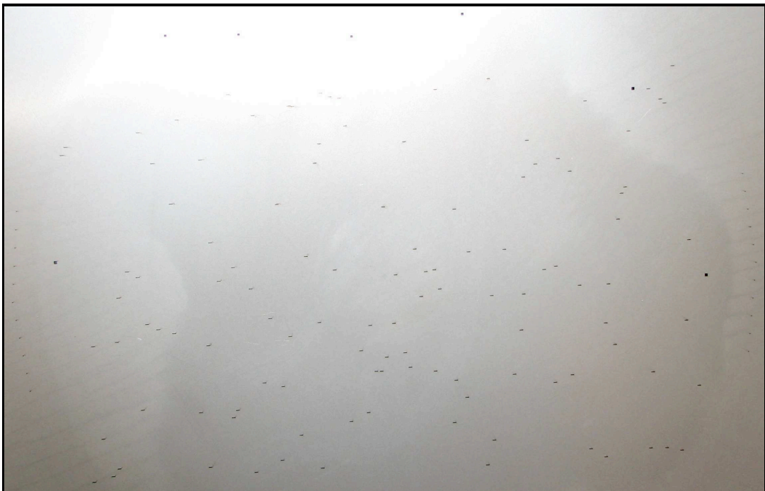
Figure 3.2: Photographs of a Multi-Slit mask. The upper panel is a photograph of a multi-slit mask resting comfortably in an armchair. The lower panel is a close-up photograph of the center of the same mask. Many slits can be seen along with several alignment boxes along the top of the photograph. The stainless steel masks are 26 inches in diameter and 0.010 inches thick.
