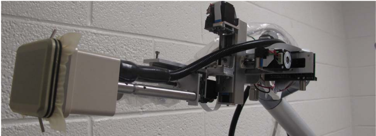
Figure 6-23: Complete integrated probe mounted to the 3 axis micro-positioner at the end of the macro-positioning arm.
