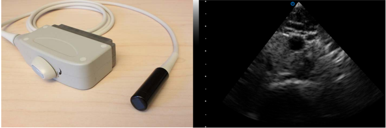
Figure 6-20: Image of the custom PA7-4 transducer (left) along with an example image taken with the transducer of the carotid artery of an adult volunteer.
