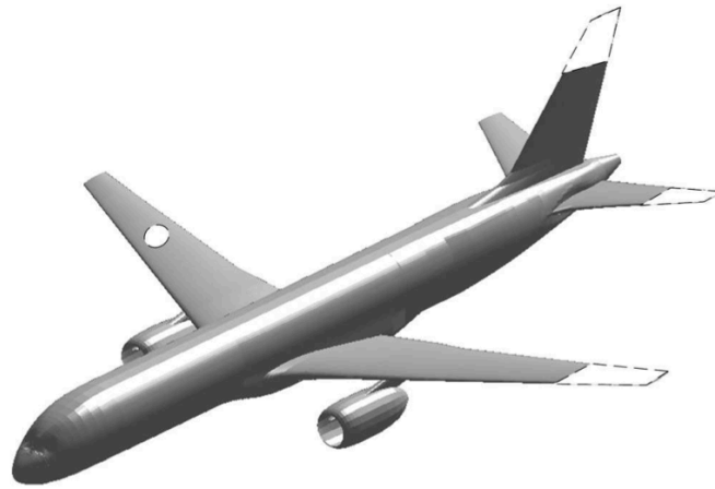
Figure 1.3: Damaged GTM (Nguyen et al. (2006)).
