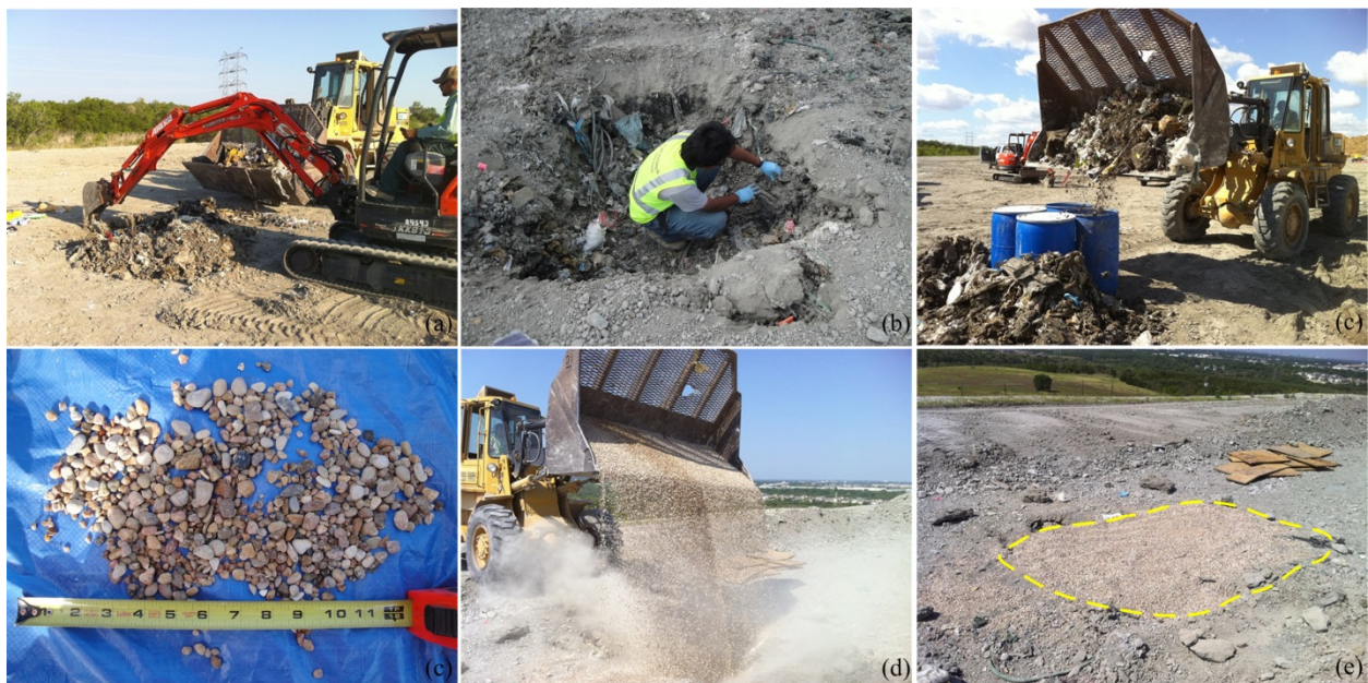
Figure 5.11 (a) Waste excavation, (b) in-situ waste characterization, (c) waste sampling, (d) pea gravel, and (d and e) in-situ unit weight measurement at the ACL.
