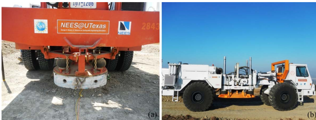
Figure 8.58 Steady-state dynamic testing using (a) Thumper and (b) T-Rex at the BKK.
