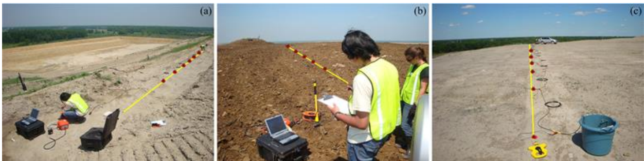
Figure 3.13 Surface wave testing at the Carleton Farms Landfill: (a) location 1, (b) location 2, and (c) location 3.
