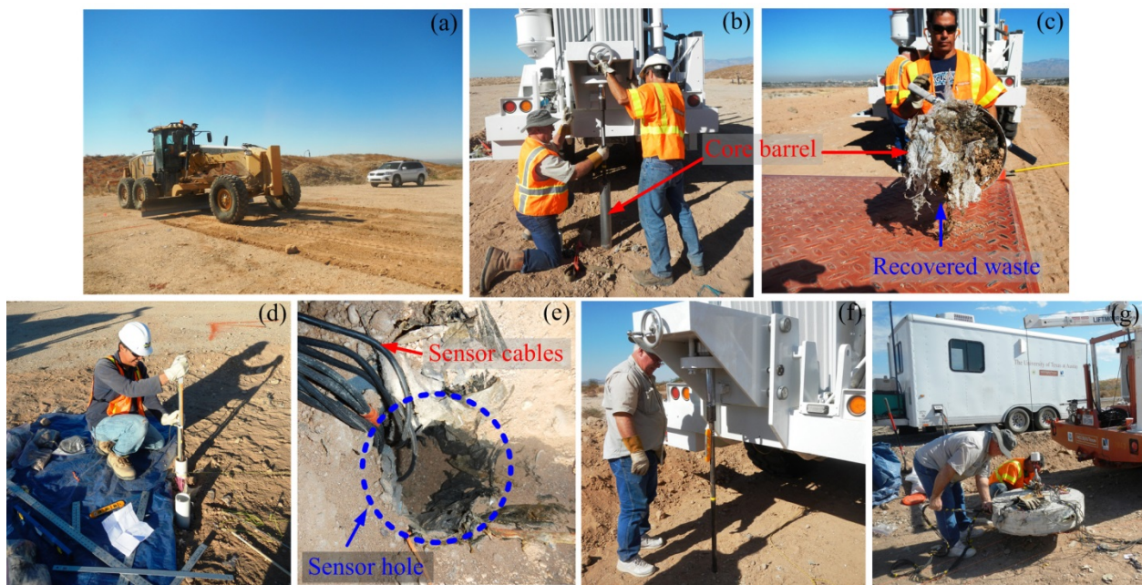
Figure 7.6 Field instrumentation and testing setup at the LRL: (a) removing cover soil, (b) pushing core barrel, (c) recovered waste from core barrel, (d) 3-D geophone installation, (e) sensor hole, (f) crosshole source rod installation, and (g) footing placement.
