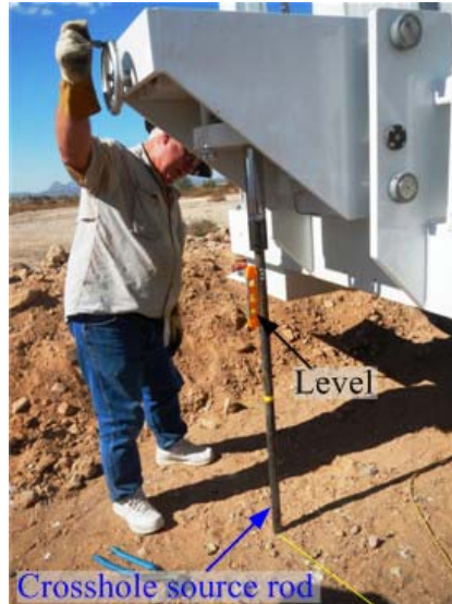
Figure 4.11 Installation of crosshole source rod.
