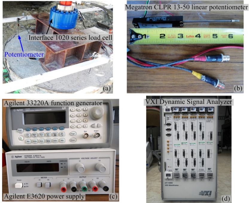
Figure 4.5 (a) Load cell, (b) linear potentiometer, (c) power supply and function generator, and (d) dynamic signal analyzer used in the field test.
