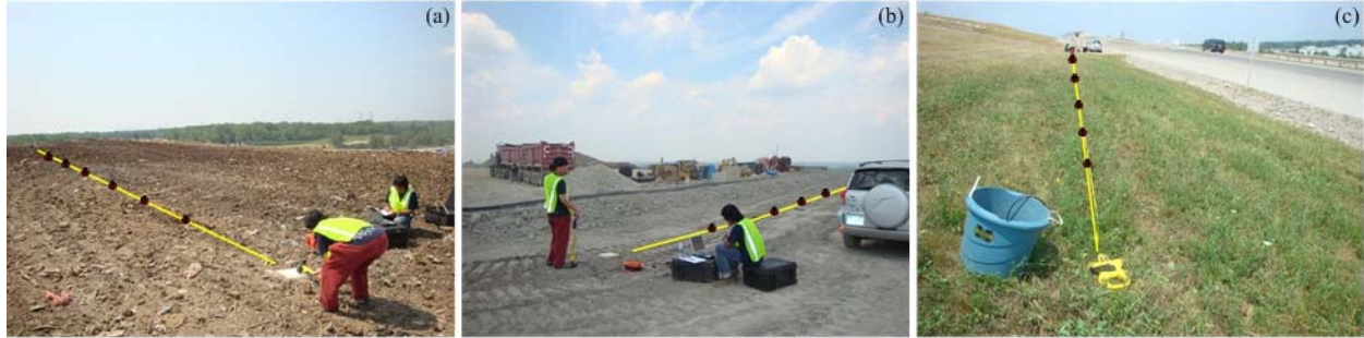
Figure 3.16 Surface wave testing at the Sauk Trail Hills Landfill: (a) location 1, (b) location 2, and (c) location 3.
