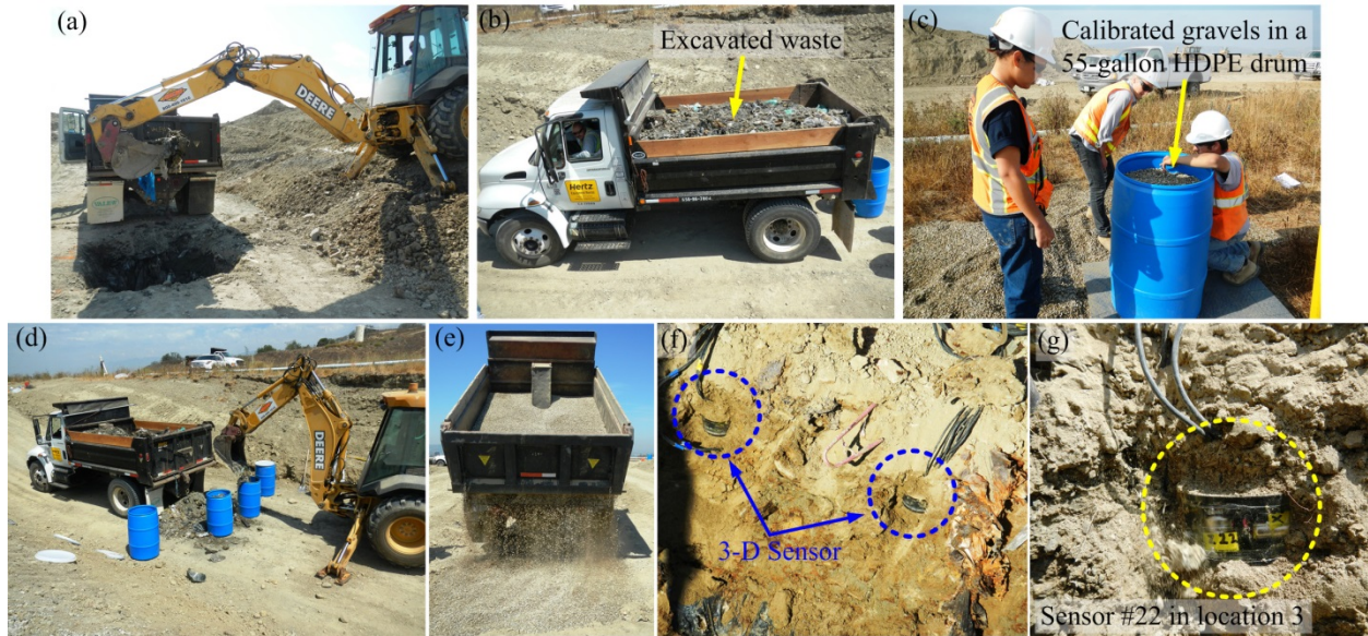
Figure 8.11 (a) Waste excavation, (b) excavated waste in the dump truck, (c) calibrated gravels in a 55-gallon HDPE drum, (d) placement of waste into drums, (e) in-situ unit weight measurement, (f) an exposed 3-D sensor pair, and (g) an exposed 3-D sensor in location 3.
