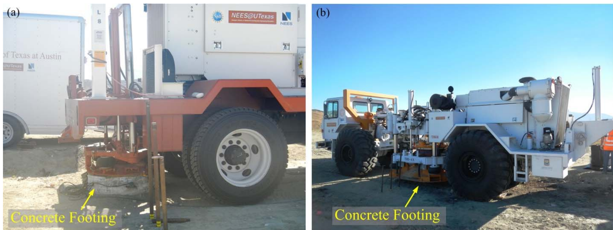
Figure 6.55 Steady-state dynamic testing using (a) Thumper and (b) T-Rex at the LCSL.
