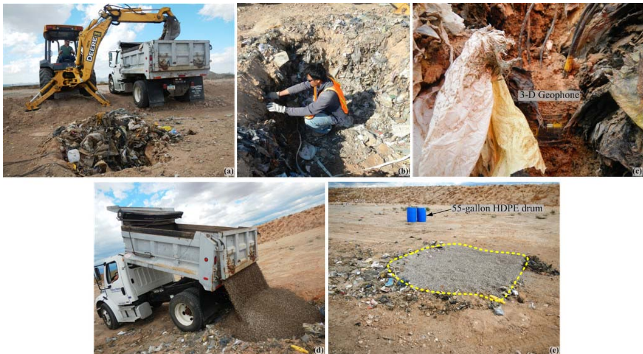
Figure 4.15 (a) Pit excavation, (b) in-situ waste characterization, (c) exposed 3-D geophone, (d) gravel backfilling, and (e) pit with gravel.
