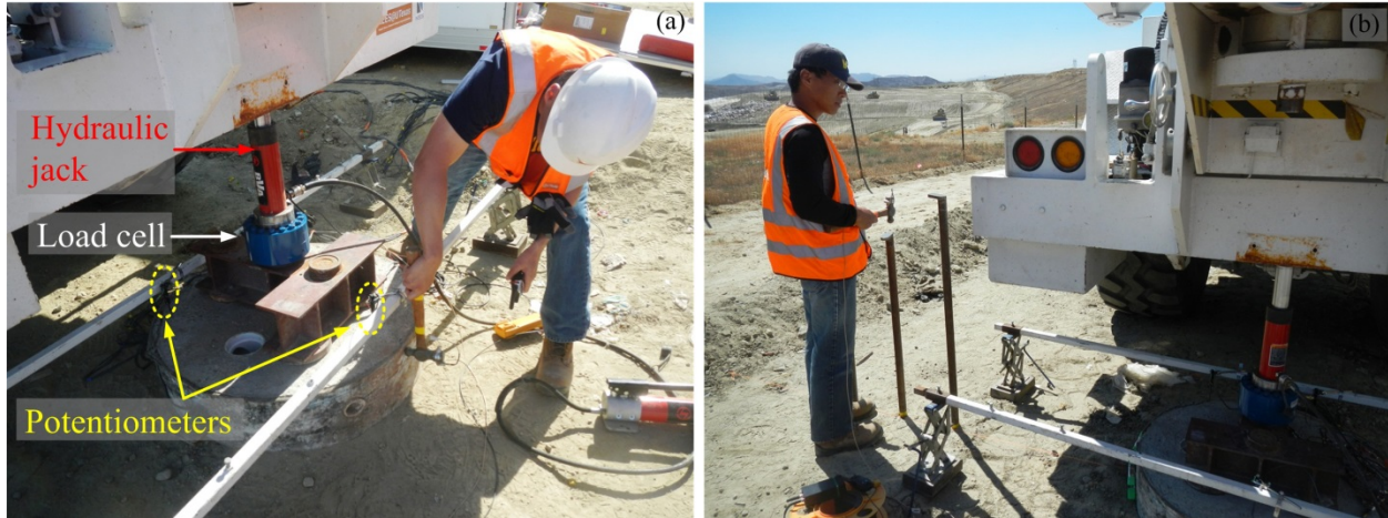
Figure 6.16 (a) Downhole and (b) crosshole seismic testing at the LCSL.
