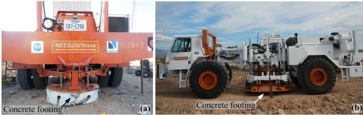
Figure 4.14 Steady-state dynamic test using (a) Thumper and (b) T-Rex.
