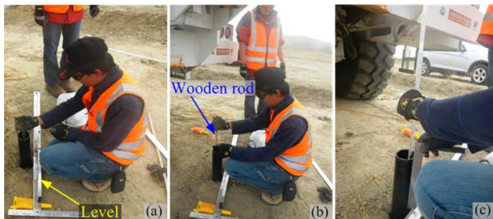
Figure 4.9 (a) Filling the borehole with fine fraction of solid waste, (b) tamping with wooden rod, and (c) checking the depth of borehole.
