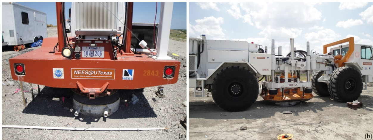
Figure 5.49 Steady-state dynamic testing using (a) Thumper and (b) T-Rex at the ACL.
