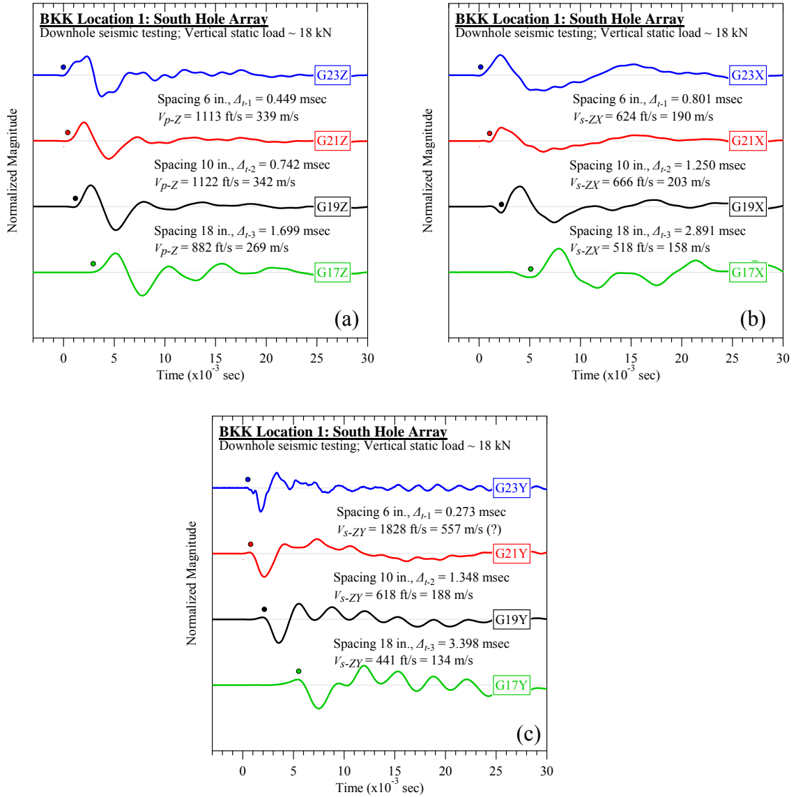
Figure D-9. BKK Landfill #1 (south hole): Downhole seismic testing at vertical load of 18 kN: (a) V_{p-Z} , (b) V_{s-ZX} , and (c) V_{s-ZY} .
