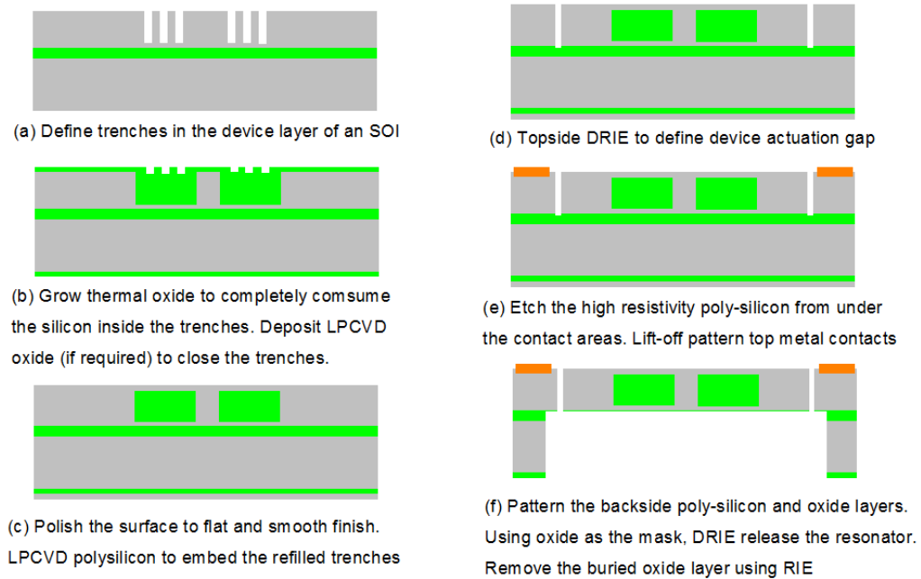
Figure 4-11: Fabrication process flow for the temperature-compensated Lamé-mode resonators.
