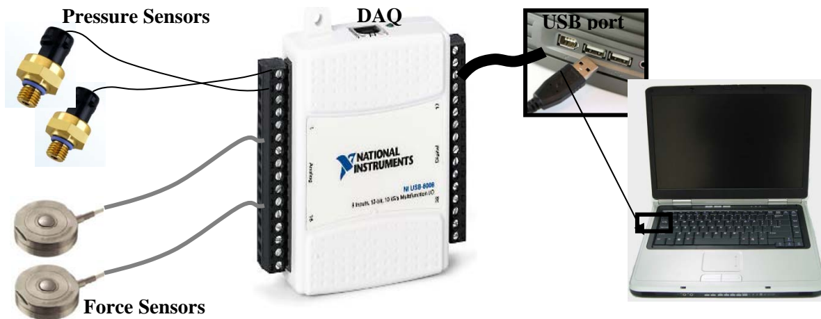
Figure 20: Physical Connectivity of System
