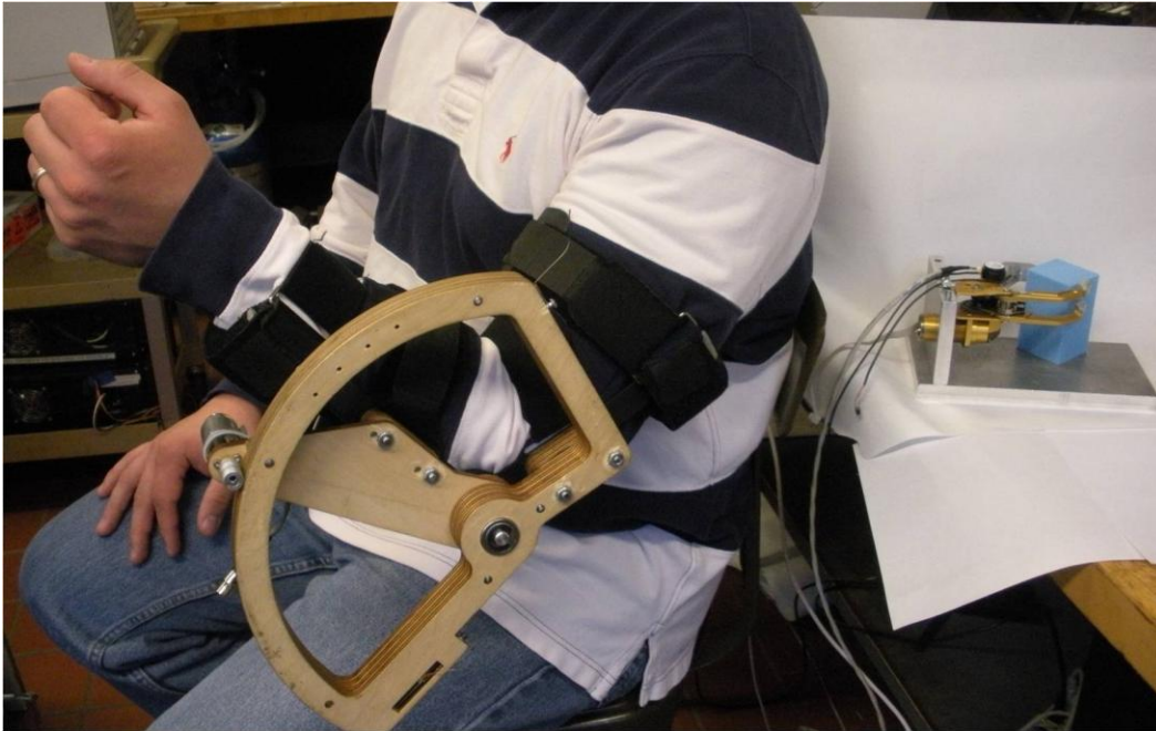
Figure 27. Entire experimental setup. The user is isolated from the terminal device controlled by EMG signals. The force and position sensing signals at the gripper are processed and then relayed back to the user by the haptic display brace.
