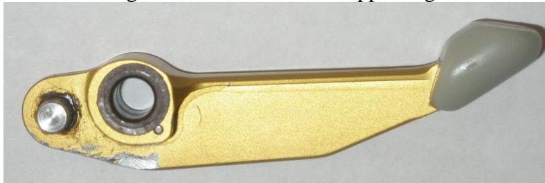
Figure 9. Disassembled Gripper Digit
