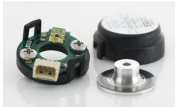
Figure 6. Rotary Optical Encoder
