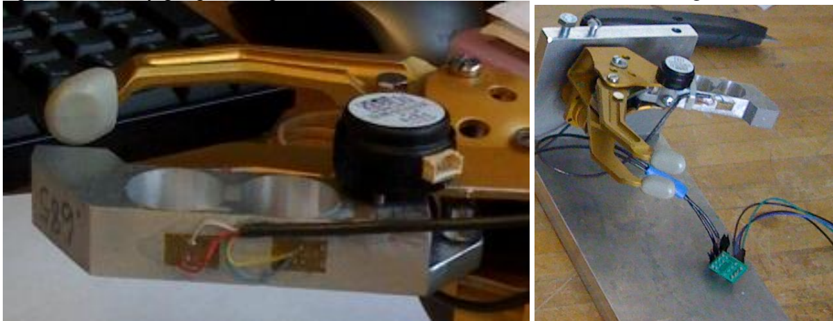
Figure 23. Vishay gauges using mounted, wire soldered, and Wheatstone Bridge assembled.
