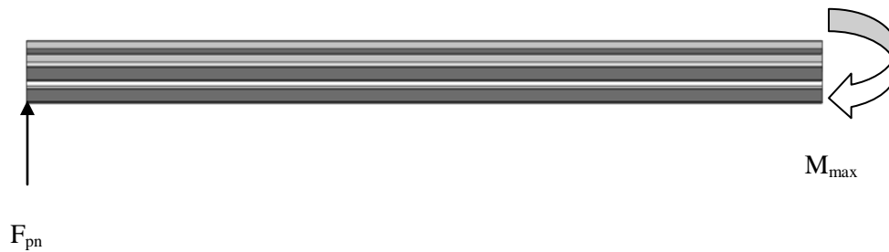
Figure I.2 Free body diagram of the cross beam
