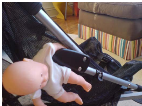
Figure 2. Dangerous pinch point in recalled MacLaren stroller [2]
