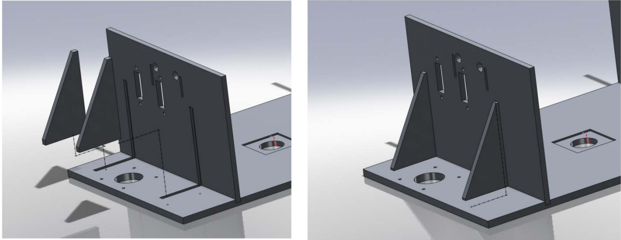
Figure 6.3: Side Reinforcement Assembly
