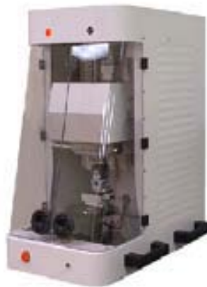
Figure 6: The most feasible currently available tribometer is the CETR-UMT tribometer capable of path generation in any 2D configuration [7]
