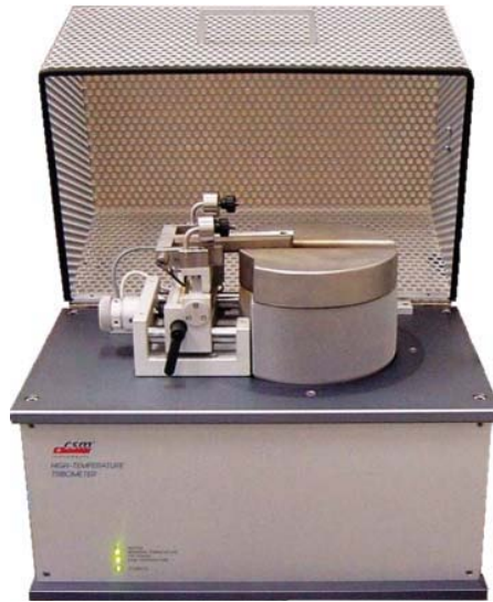
Figure 5: CSM Tribometer for linear and Rotational Testing with Environmental Enclosure [6]
