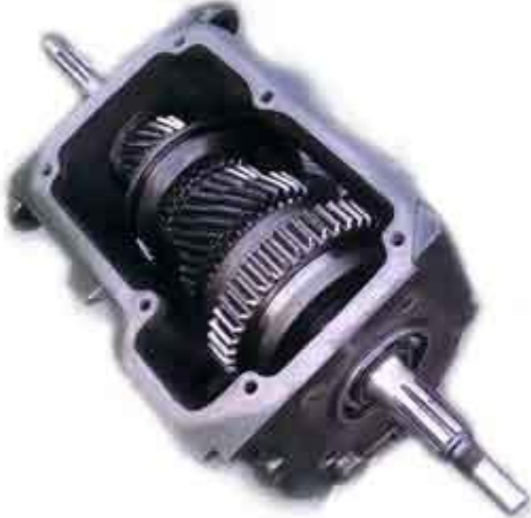
Figure 10: Example of a Gearbox
