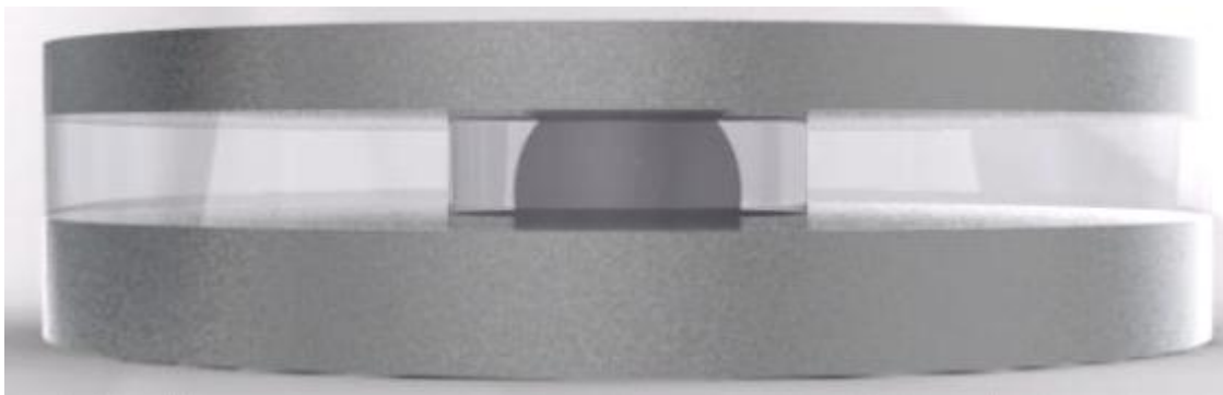
Figure 16: Ball Joint and Two Plates for x-y Plane Alignment
