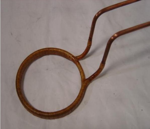
Figure 24: Resistive Heat Coils
