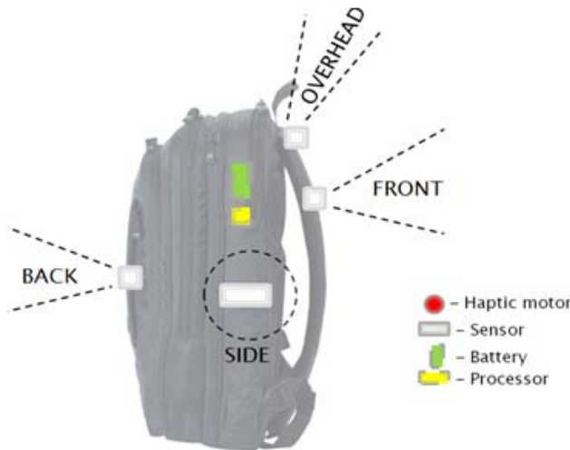
Fig 6: Layout Drawing of Backpack – Side View
