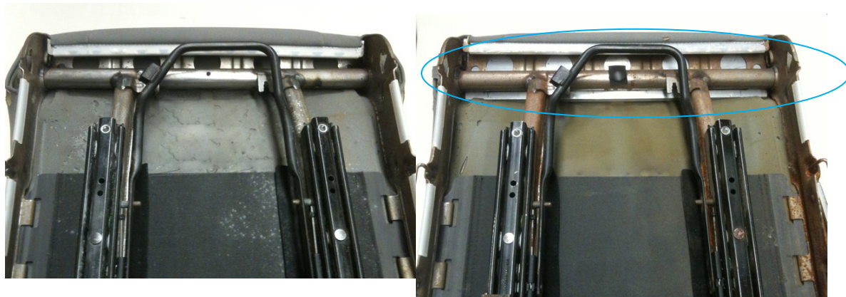
Figure 7. Standard seat cushion structure (left) and addition of aluminum plate to increase stiffness (right)
