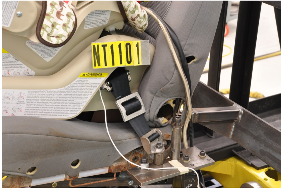
Figure 4. Close-up of inboard anchorage hardware including simulated buckle stalk
