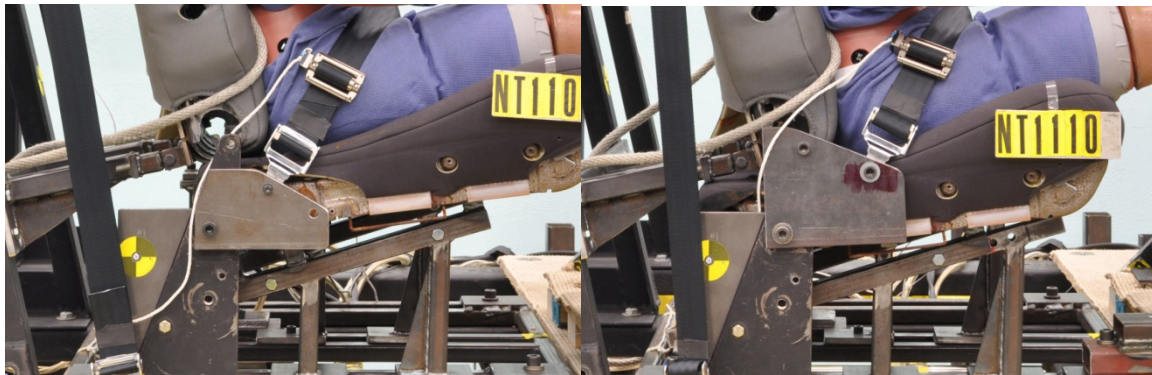
Figure 3. Mid lap belt geometry hardware (left) and optimized 6YO hardware (right)
