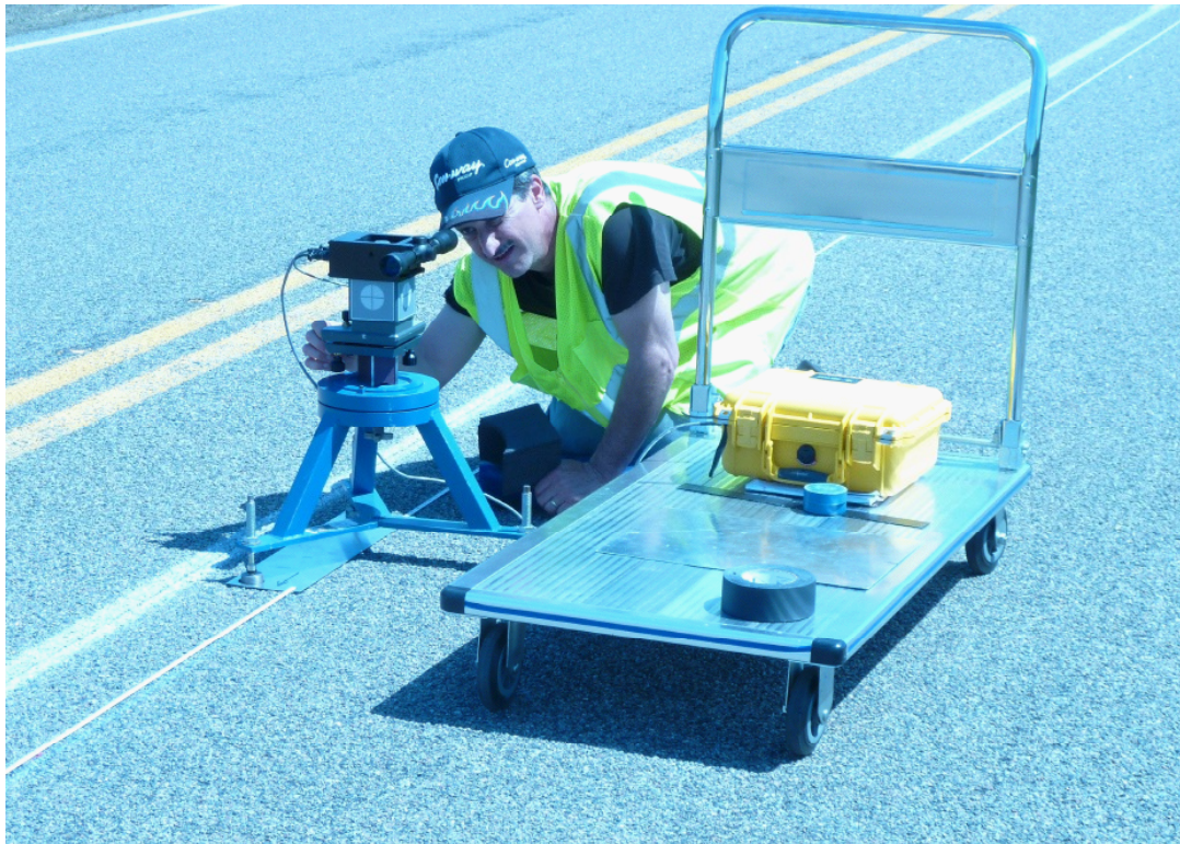
Figure B–11. Benchmark Profiler reference laser alignment.
