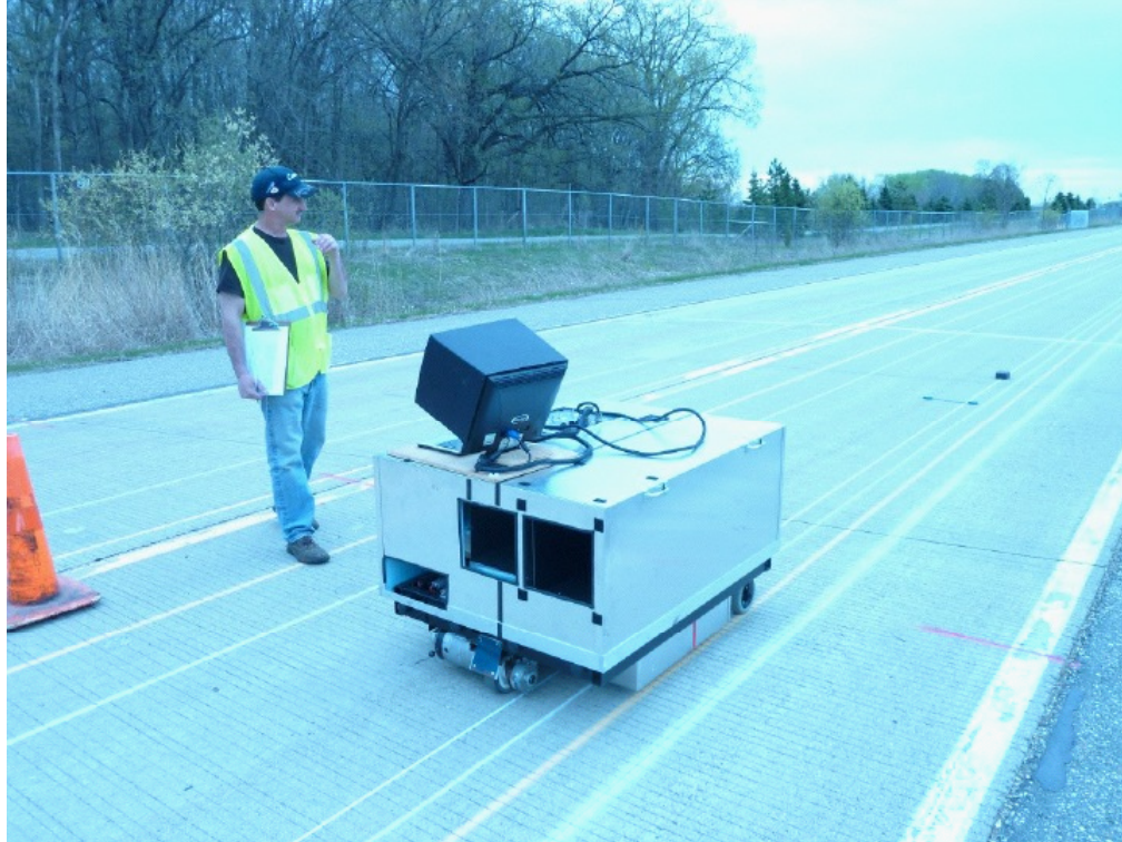
Figure B-12. Benchmark Profiler cart on the transverse tining section.
