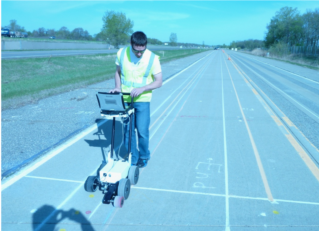
Figure B-3. SSI SC8800 Walking Profiler on transverse tining.
