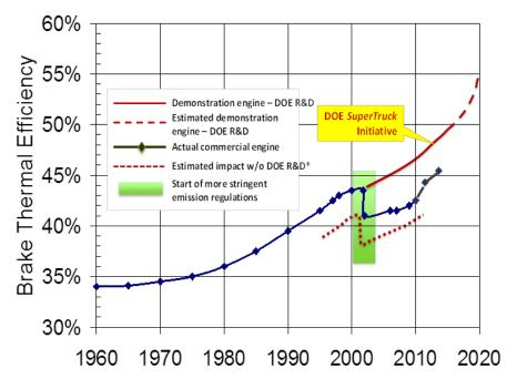
Figure 8. Historical trend in heavy-duty diesel engine efficiency (DOE, 2014).
