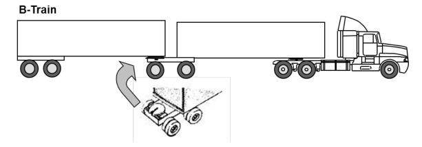
Figure 10. Illustration of Canadian B-train configuration (TAC, 1986).
