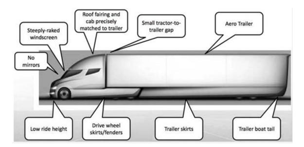
Figure 7. Aerodynamic concept presented by Oehlerking (2013).
