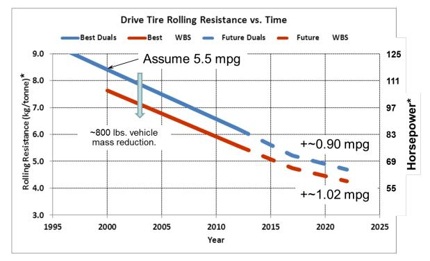
\* Note: Values represent the evolution of the lowest rolling resistance long-haul drive tires. Other performance is assumed equivalent. Absolute values depend on test equipment and conditions. Actual values in the market will vary. Horsepower represents consumption due to tires at 65 mph, 80,000 lb total load.
