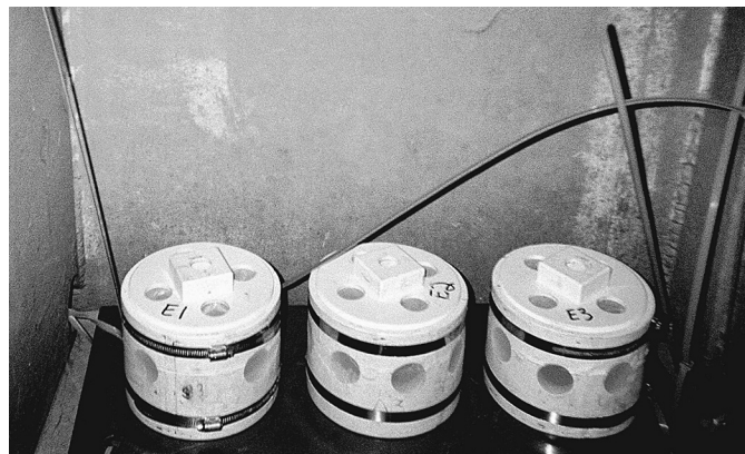
Fig. 1. Polyvinyl-chloride incubation chambers installed in an empty ballast tank. Side and top windows were covered in 60- \mu m nitex mesh. Inner diameter of chambers is 15 cm.
