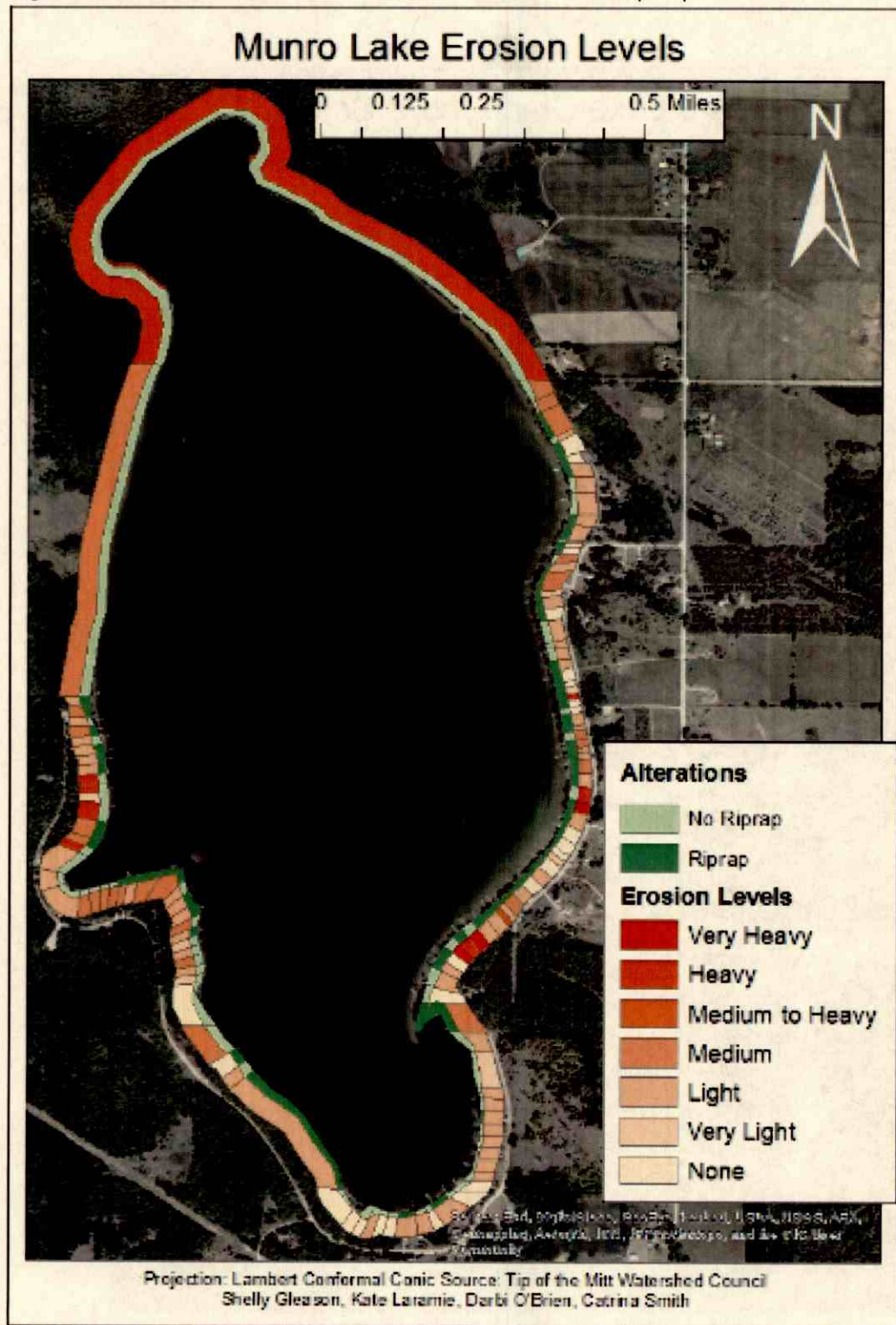
Figure 4. Erosion levels and alterations with or without rip-rap
