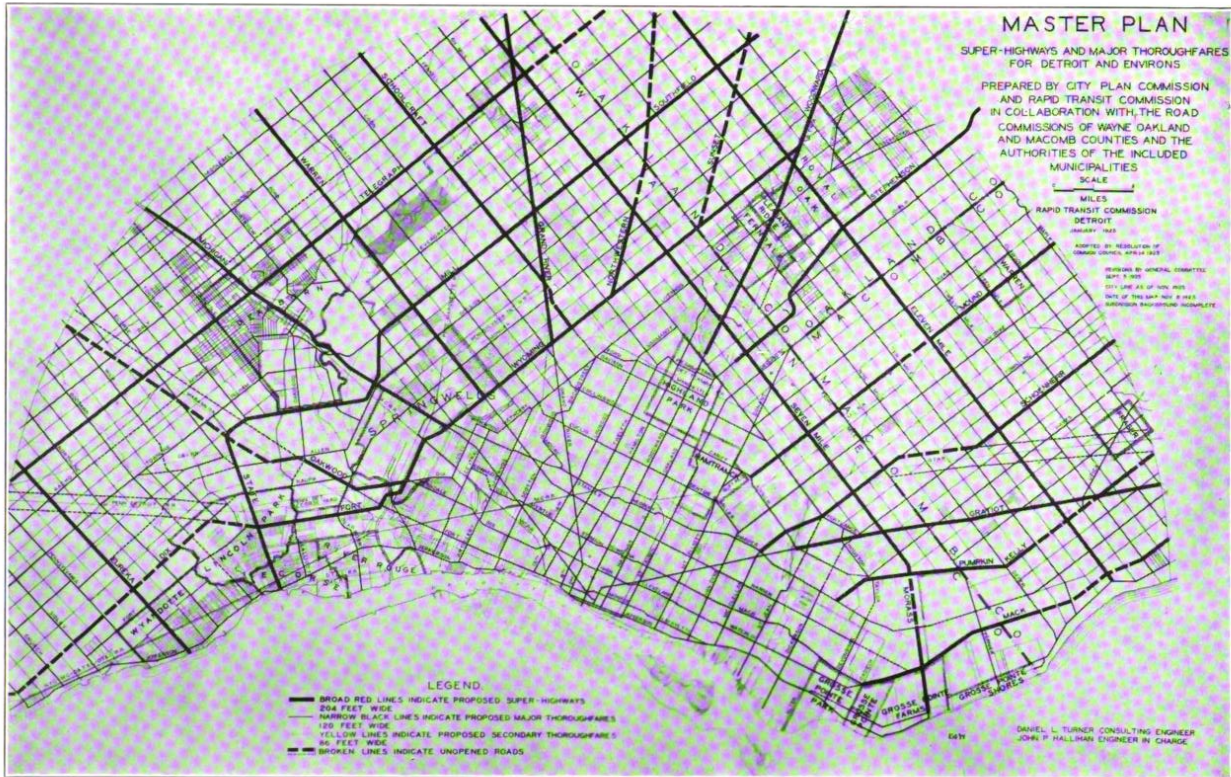
Figure 70. Master Plan of super-highways and major thoroughfares for Detroit and environs, January 1925. Superhighways shown in thick black lines, thoroughfares in thin black lines.
