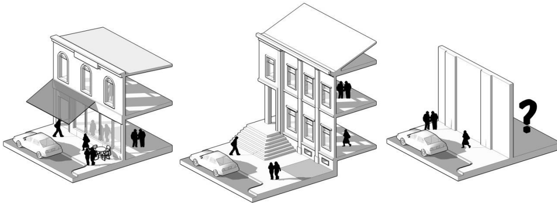
Figure 16. Commercial functions (left) are highly interactive and propel an image of low ‘threshold resistance’, while institutional buildings (middle) may aim for more exclusivity. Blank walls (right) completely shield public from private space. 158
