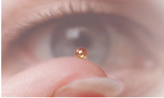
Figure 1.6: An ICF fuel pellet. The pellet consists of a thin, spherical plastic shell filled with a mixture of the hydrogen isotopes deuterium and tritium. Photo credit: LLNL Science and Technology Review [30]
