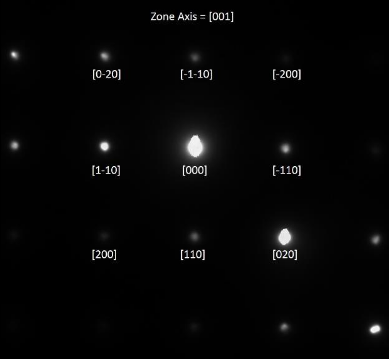
Figure 4.44 Diffraction pattern of the bcc crystal lattice from the \langle 100 \rangle zone axis taken from an irradiation creep sample.
