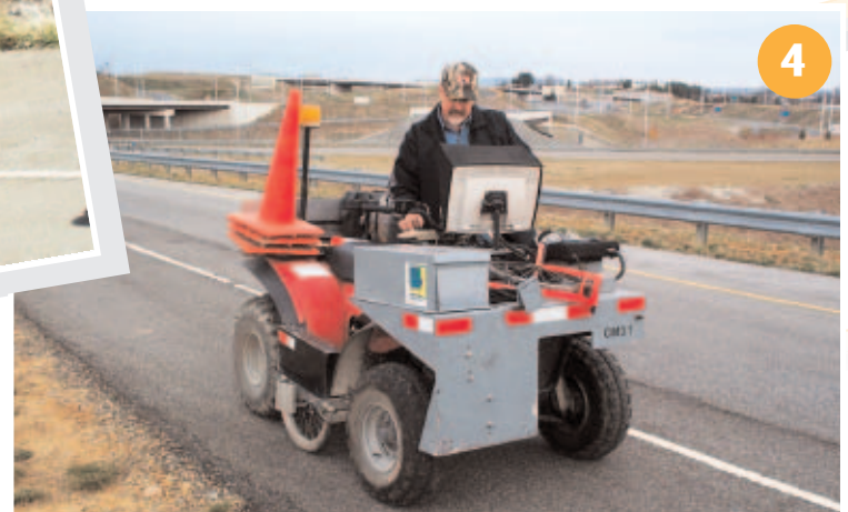
Some of the equipment tested at the roundup event included (top to bottom): (1) a custom-built profiler owned by the Federal Aviation Administration; (2) the ROMDAS Z-250 roughness calibration profiler, operated by Jerry James; (3) the Auto Rod and Level, built by APR Consultants, Inc. and operated by Mike Freeman (left) and Tony Gerardi; and (4) the ICC lightweight profiler, owned by New Enterprise Stone & Lime Co., Inc. and operated by Ed Wilson.
