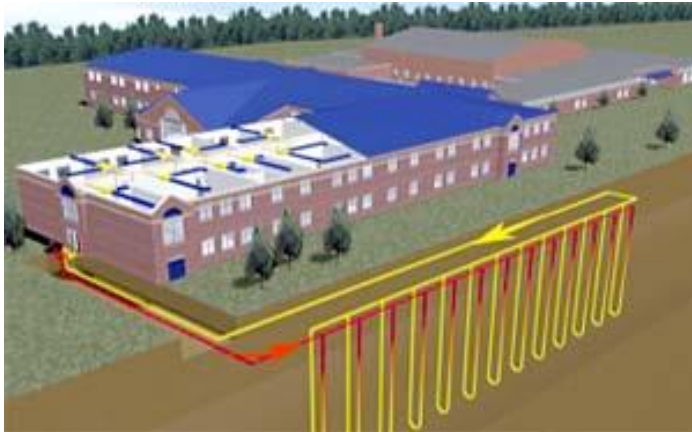
Figure 22. Geothermal Heating and Cooling of a School
