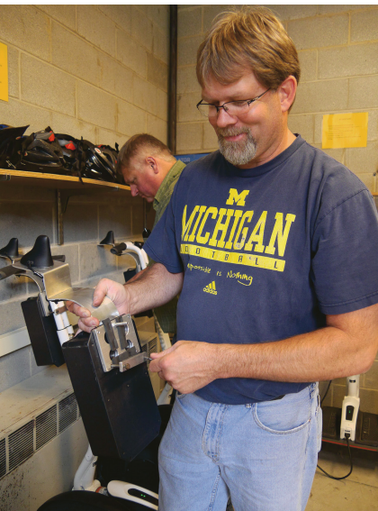
UMTRI technicians Ken Winzeler (front) and John Koch install V2V communication devices on Segways.
