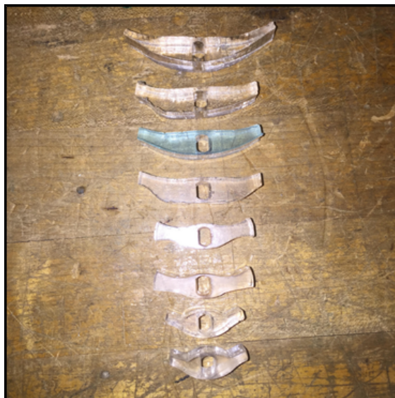
Fig 13.1.1: From bottom to top, the design of the valve has changed as the horizontal length highly affects the length of our stride as well as how long the swinging leg is actually raised.
