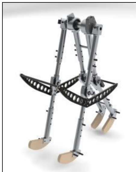
Fig 2.1 The above walker (Derek Coop, U. of Manitoba [7]) resembles a double pendulum. Given appropriate initial conditions, it will exhibit dynamic behavior that resembles human walking.
