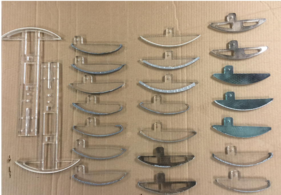
Figure 14.2.2: The various foot profiles which were empirically tested on our walker. The optimized foot profile is shown on the walker itself in figure 14.2.1.
