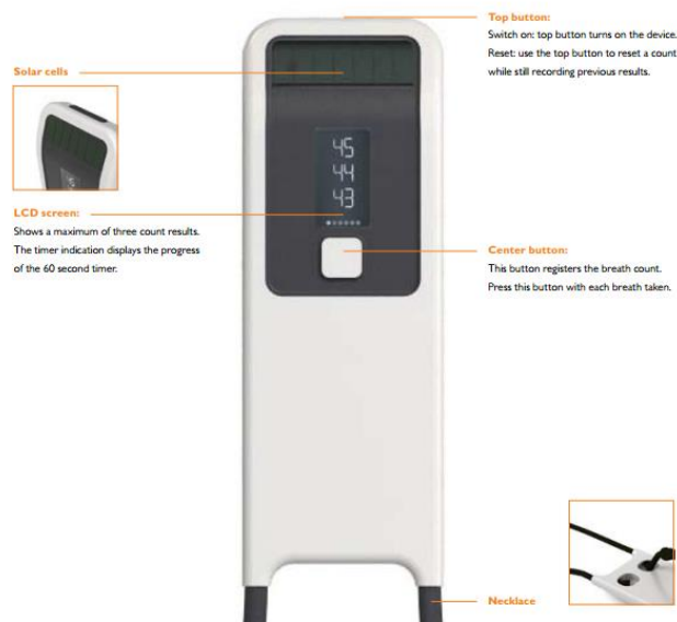
Figure 3: Conceptual breath counter designed by Phillips featuring; an LCD screen which displays the count result and timer, solar cells, input button, and neck strap [6].
