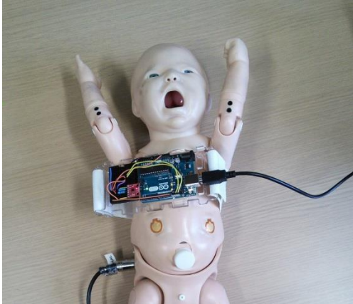
Figure 11: Validation testing was performed on a high-fidelity infant simulator. Respiratory rate was set and compared to the rate calculated by the device.
