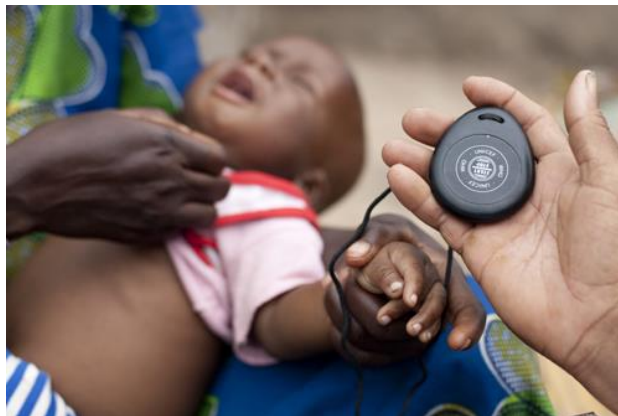
Figure 1: The Acute Respiratory Timer keeps track of time over 60 seconds, while the caregiver visually counts each breath the child takes [5].
