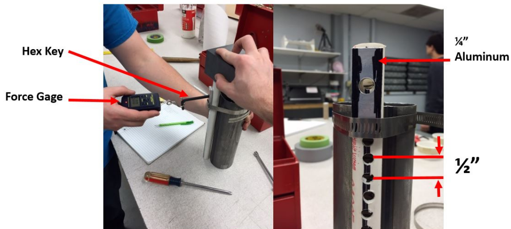
Fig. 42: The test procedure for the trigger force experiment can be shown in this series of photographs.
