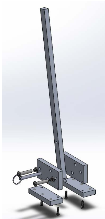
Figure C.7: Exploded view of lever assembly
