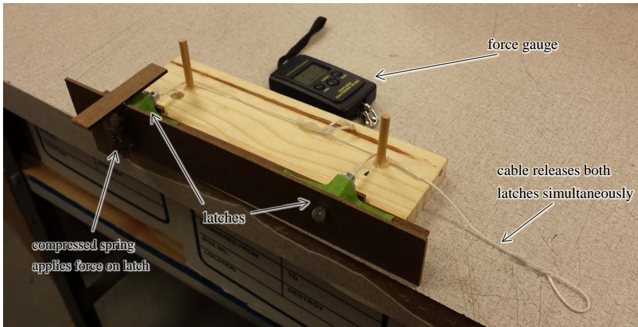
Fig. 44: Testing rig for difference in latch release behavior
