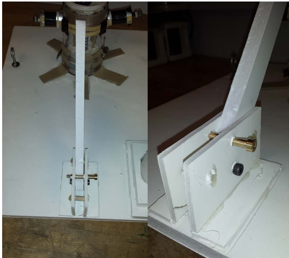
Fig. 45: The lever mechanism consists of a base and a lever arm. To prevent accidental launch, a pin is inserted to act as a hard stop. It is inserted through the base to prevent the lever from being pulled. This is simple and will ensure that the pin safety will be used every time.
