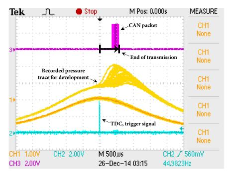
**Figure 7.5** This figure shows an infinite persistence oscilloscope trace for verifying CAN packet latency constraints are met.
