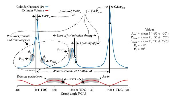
**Figure 3.1** A schematic of key engine cycle variables. The timing of both  $P_{IVC}$  and  $P_{NVO}$  have been modified from the original version in [41] to meet real-time engine controller timing requirements.  $P_{IVC}$  was moved to the previous cycle and  $P_{NVO}$ 's crank angle range was shortened.  $P_{IVC}$  has also been moved closer to TDC to take advantage of the inherent signal amplification provided by the compression process.
