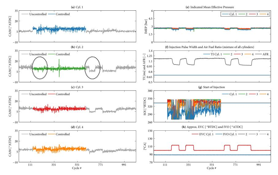
**Figure 8.5** Controller performance at 2,500 rpm with large Exhaust Valve Close (EVC) steps from 100 to 113  $^{\circ}$ BTDC, see subplot h. At this operating point, this was the largest open loop EVC step possible. Cylinder 2 remains in a region with the most SOI control authority (away from the lower SOI limit), and thus its performance is highlighted with the dashed ovals.
