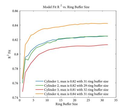
**Figure 6.5** Ring buffer size sensitivity with 64 neuron WR-ELM and  $W_0 = 3.5 \times 10^{-3}$ .
