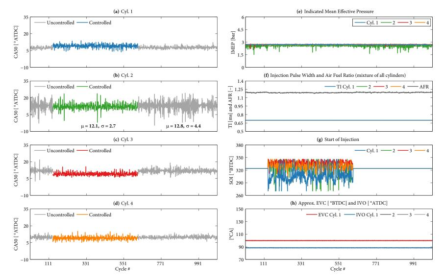
**Figure 8.7** Controller performance for reducing cyclic variability on cylinder 2 while maintaining a combustion phasing similar to uncontrolled mean value at 2,500 rpm.
