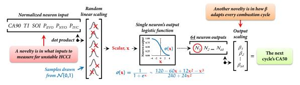
Figure 4.1 A graphical schematic of the Extreme Learning Machine used in this work.
