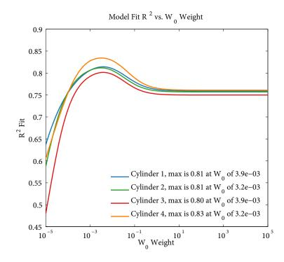
**Figure 6.1**  $W_0$  sensitivity with 64 neuron WR-ELM and ring buffer size of 8.
