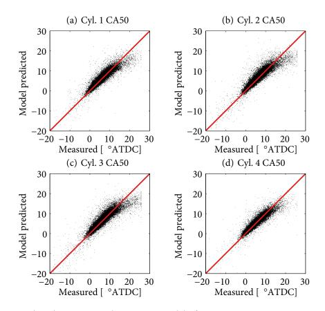
**Figure 5.5** Predicted vs. measured WR-ELM model of Eq. 3.14 across 25,323 consecutive cycles with random transient steps occurring approximately every 0.5 - 10 sec. and occasional misfires. Late phasing is somewhat under predicted, but almost all prediction outliers still capture the correct directionality.
