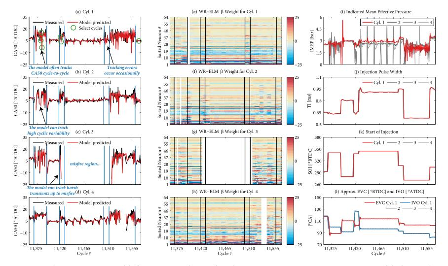
**Figure 5.6** The WR-ELM CA50 model of Eq. 3.14 can track CA50 through transients every 0.5 - 10 sec., operating points with high CV, and at steady-state during a particularly harsh region of the 25,323 cycle dataset that includes misfires. The colormaps (linearly scaled) provide qualitative insight into the level of cycle-to-cycle adaptation and into cylinder-to-cylinder model differences. The blue and black vertical lines mark random engine set point steps in sub-figures a-h.
