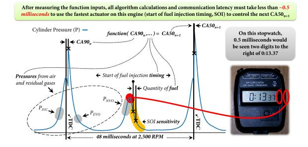
**Figure 7.2** Using SOI as a real-time control actuator with the prediction algorithm requires tight computational latency constraints to be satisfied. The stopwatch image has been released into public domain [60].
