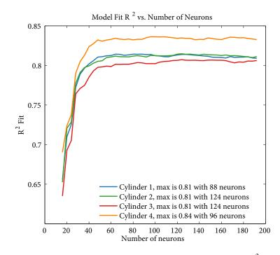
Figure 6.4 Model sensitivity to the number of neurons with  $W_0 = 3.5 \times 10^{-3}$  and a ring buffer size of 8
