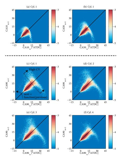
**Figure 5.2** Experimentally acquired return map probability histograms of CA10, CA50 and CA90 using the 129,964 cycle dataset with 2,221 actuator set points. The colormap is log<sub>10</sub> to show order of magnitude differences.
