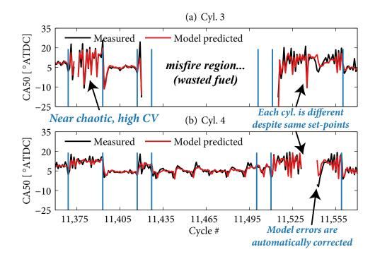
**Figure 9.1** Multi-cylinder predictions with the techniques developed in this dissertation. Each blue vertical line is a harsh, simultaneous transient of four different engine actuators (see Fig. 5.6 for detailed information about the actuator settings).
