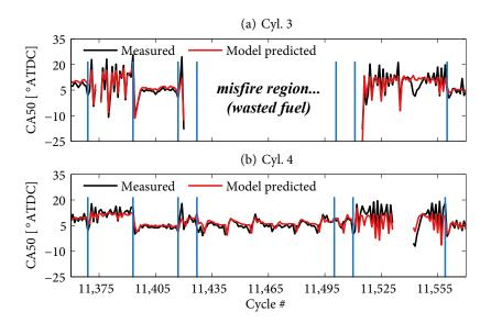
**Figure 6.3** Model performance with  $W_0 = 3.5 \times 10^0$  and a ring buffer size of 8.
