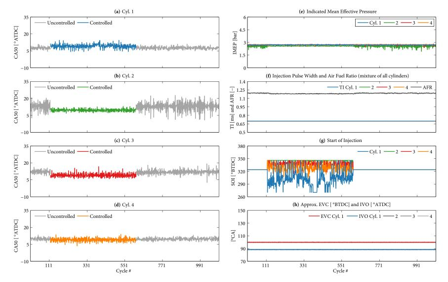
Figure 8.3 Control enabled to balance cylinders to a similar combustion phasing at 2,500 rpm.
