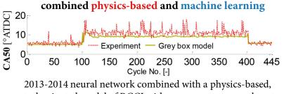
control-oriented model of RCCI with over an octane number step.
