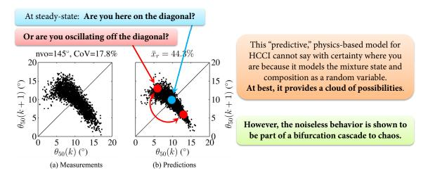
**Figure 1.3** Steady-state simulations of combustion phasing at the combustion stability limit with residual fraction noise to capture CV. Adapted from [8] under fair use.
