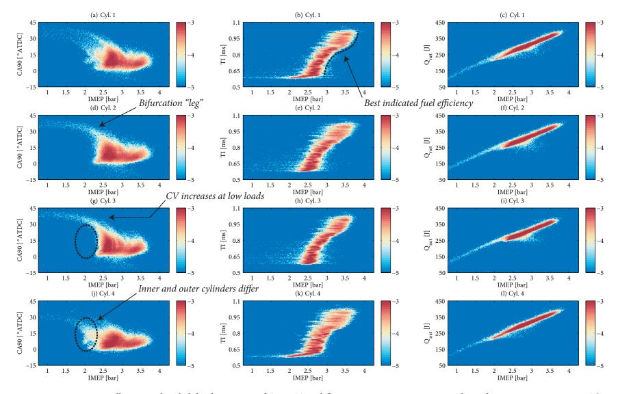
**Figure 5.3** Experimentally acquired probability histograms of CA90, TI and  $Q_{net}$  vs. IMEP across 129,964 cycles and 2,221 actuator set points. The colormap is  $\log_{10}$ .
