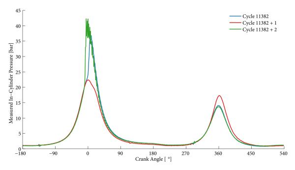
Figure 6.7 Pressure traces for the high CV cycles in Fig. 5.6(a).
