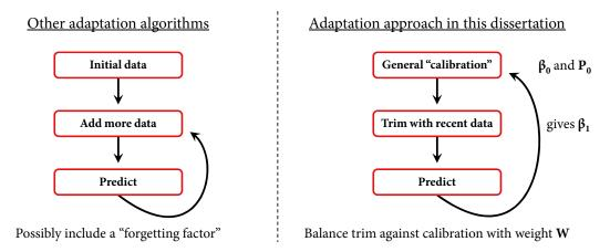
**Figure 4.3** A high-level view of how the adaptation algorithm in this dissertation differs from typical machine learning adaptation approaches.
