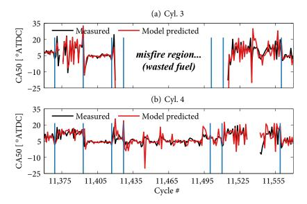
**Figure 6.2** Model performance with  $W_0 = 3.5 \times 10^{-6}$  and a ring buffer size of 8.
