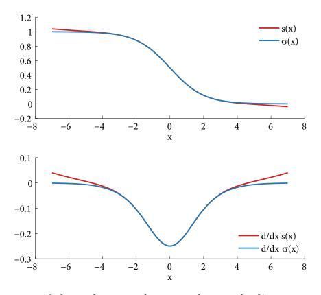
Figure 4.4 The logistic function, its derivative, and associated Padé approximations.
