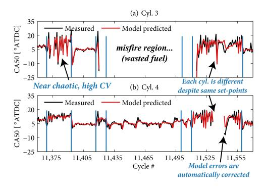
**Figure 1.6** Multi-cylinder predictions with the techniques developed in this dissertation. Each blue vertical line is a harsh, simultaneous transient of four different engine actuators (see Fig. 5.6 for detailed information about the actuator settings).
