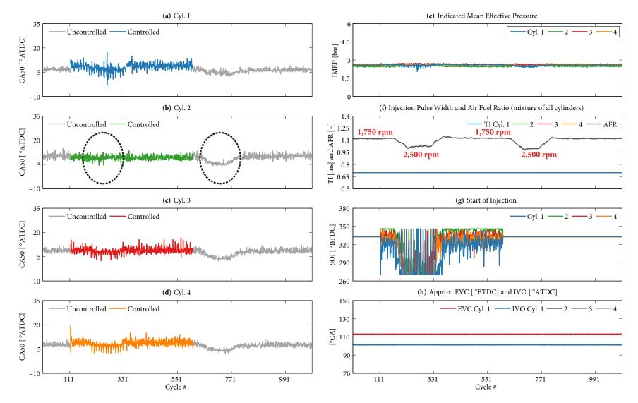
**Figure 8.6** Controller performance with large engine speed ramps from 1,750 to 2,500 rpm and back are shown in each segment. Note that there is no engine speed in this model — predictive control outside the model's original design is being achieved with adaptation. Cylinder 2 remains in a region with the most SOI control authority (away from the lower SOI limit), and thus its performance is highlighted with the dashed ovals.
