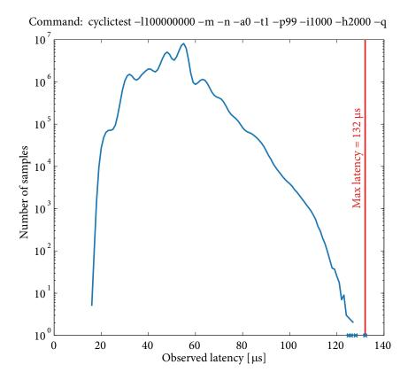
**Figure 7.3** A ~28 hour latency test while acquiring 8 simultaneous channels worth of 18 bit pressure data at 32 kHz (256 kilosamples per second, total) with the custom data acquisition hardware developed in this work, under moderate CPU load, with continuous network and SD card storage access.
