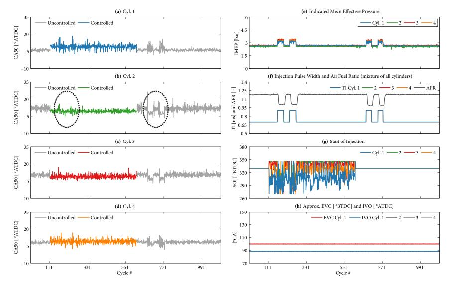
**Figure 8.4** Controller performance at 2,500 rpm with a large (29%) increase in injection pulse width (TI), see subplot f. Cylinder 2 remains in a region with the most SOI control authority (away from the lower SOI limit), and thus its performance is highlighted with the dashed ovals.
