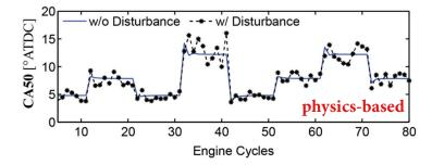
2013-2014 control-oriented HCCI model simulation where the author adds noise to model the oscillations.
