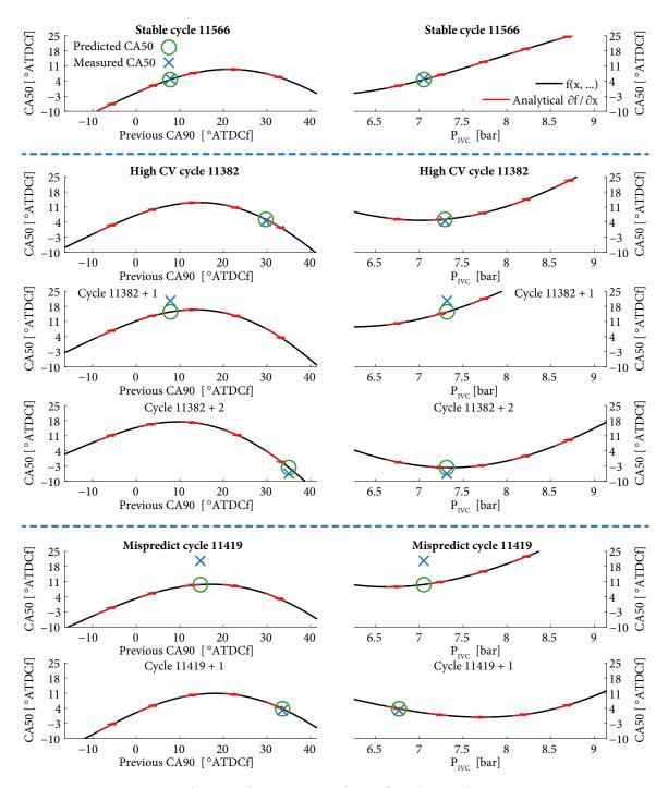
Figure 6.9 CA90 and  $P_{IVC}$  extrapolation for select cycles in Fig. 5.6(a).
