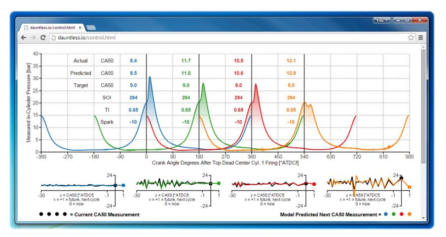
Figure 8.1 A screenshot of the custom software developed for this dissertation. Real-time predictions are shown while engine control is disabled.
