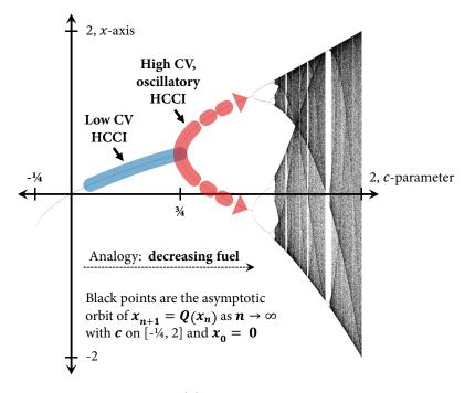
**Figure 2.1** The bifurcation diagram of Q(x) as c is varied, along with a qualitative representation of how one might view high CV HCCI.
