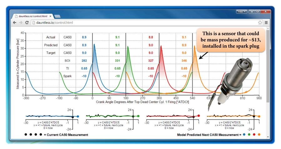
Figure 8.2 Control enabled using Eq. 8.1 for a set point of 9 °ATDC firing. The overlaid spark plug pressure sensor image was provided by Optrand<sup>®</sup> Inc.
