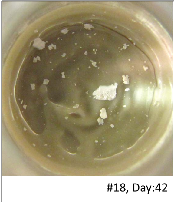
Figure 5.2 A mixture of propanol, acetone, methyl isobutyl ketone, 2-butoxyethanol, amyl acetate, and n-butyl acetate dissolved in PCE ponded on water-saturated bentonite for 42 days. No cracking was observed.
