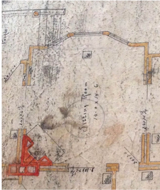
Figure 13: On this original plan P05 received from the previous owner of her house, she noticed that a wall in her house used to be a pocket door. She was able to reopen the wall to restore the doorway.
