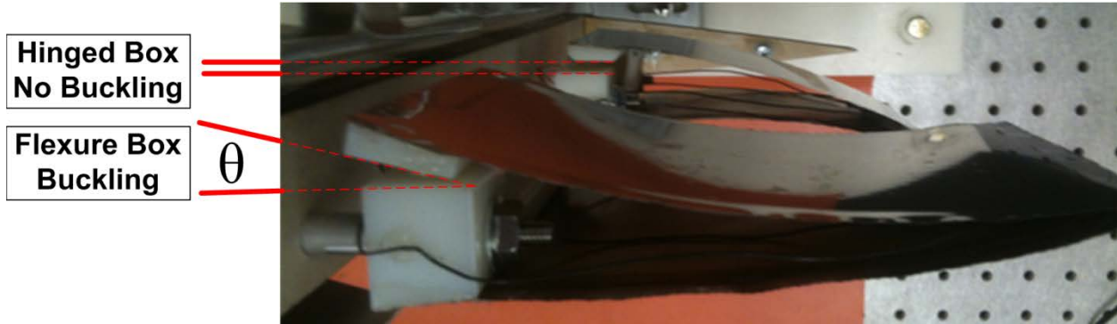
Figure 2.14 Flexure Box Buckling (foreground) and Hinged Box (background)
