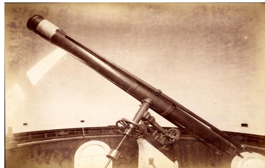
Henry Fitz refracting telescope in dome of UM Detroit Observatory, ca. 1870. From UM Photographs Vertical File.
